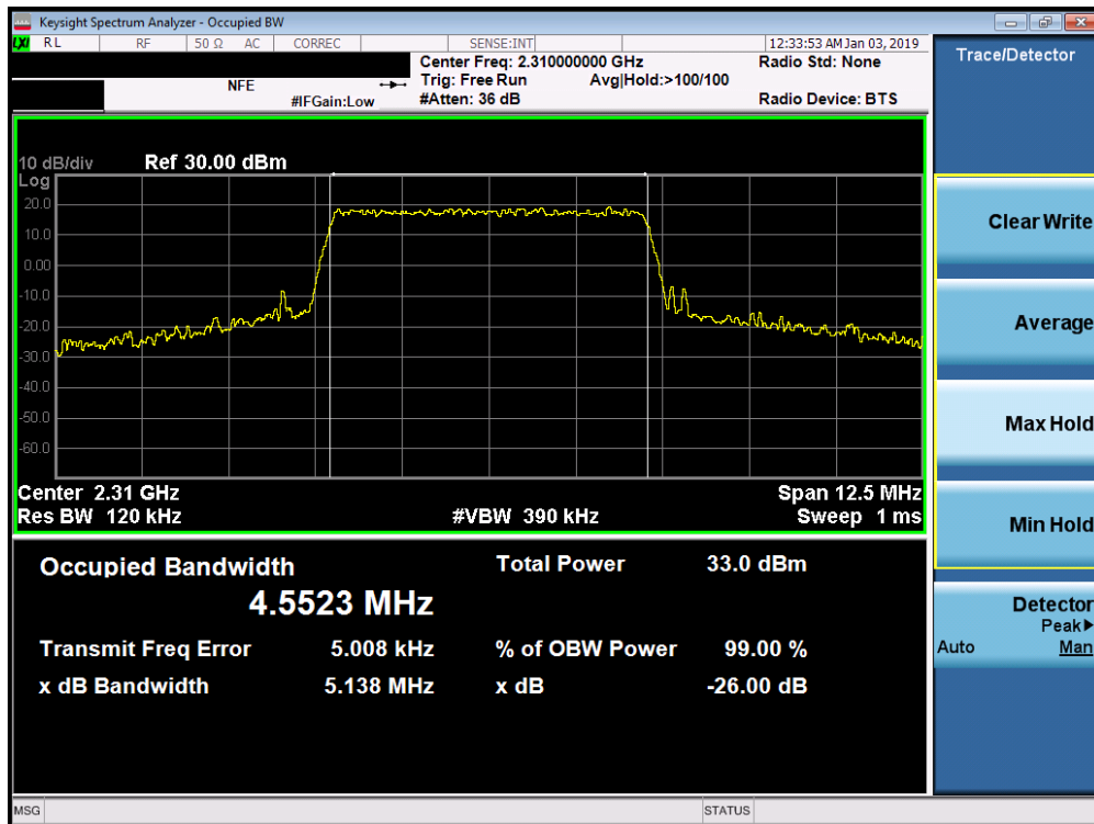
Plot 7-68. Occupied Bandwidth Plot (Band 30 - 5.0MHz 16-QAM - Full RB Configuration)
