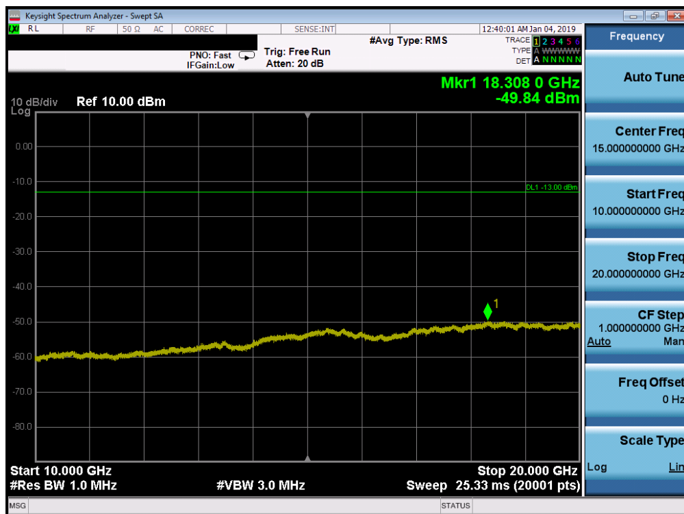
Plot 7-46. Conducted Spurious Plot (PCS WCDMA Mode - Low Channel)
