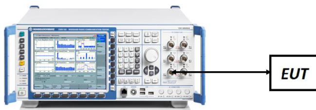
Figure 7-5. ERP/EIRP Measurement Setup
