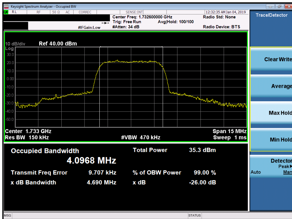
Plot 7-6. Occupied Bandwidth Plot (AWS WCDMA Mode)
