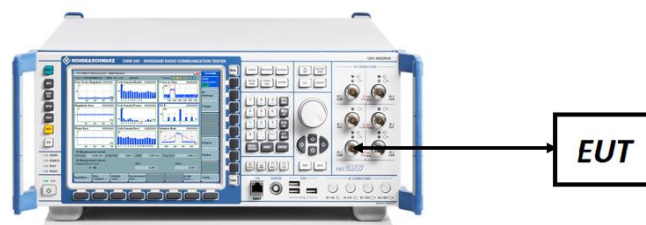
Figure 7-4. Conducted Power Measurement Setup
