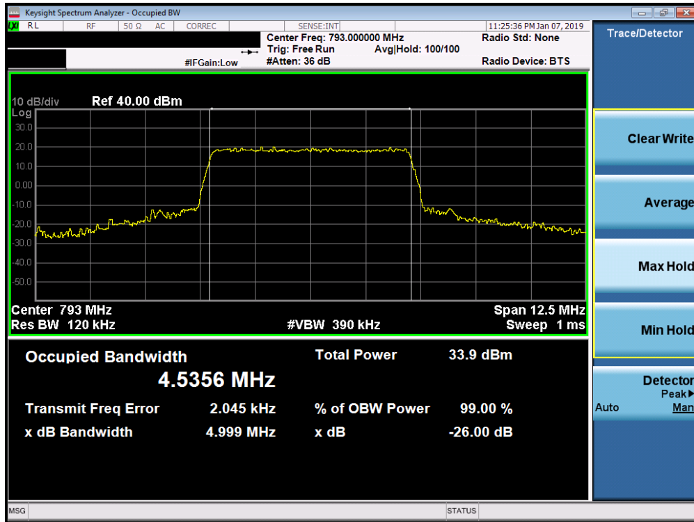
Plot 7-13. Occupied Bandwidth Plot (LTE Band 14, 5MHz QPSK – RB Size 25)
