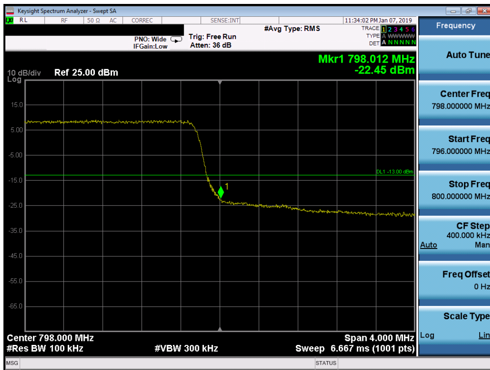
Plot 7-40. Upper Band Edge Plot (LTE Band 14, 5MHz QPSK – RB Size 25)
