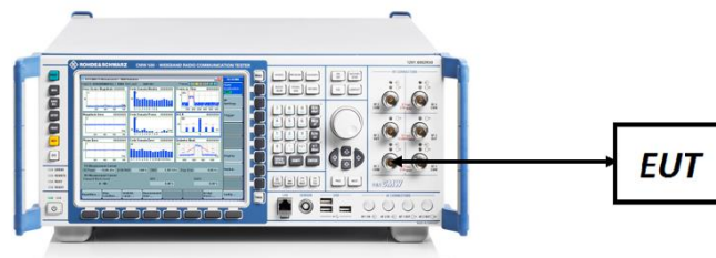
Figure 7-5. ERP Measurement Setu
