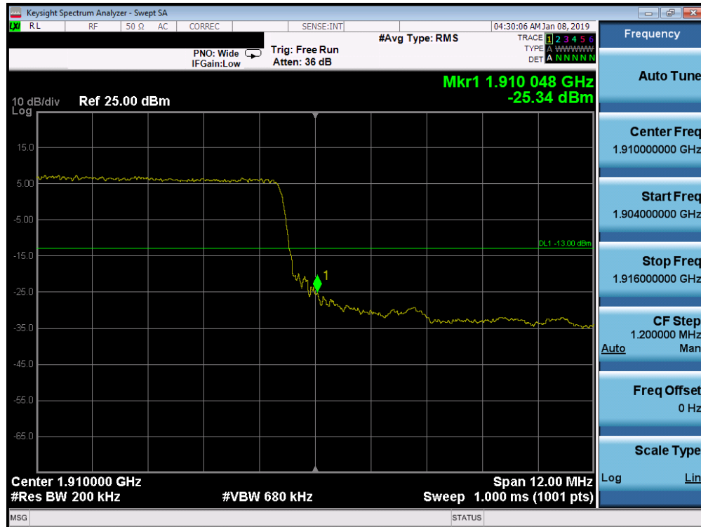
Plot 7-291. Upper Band Edge Plot (Band 2 - 15.0MHz QPSK - Full RB Configuration)
