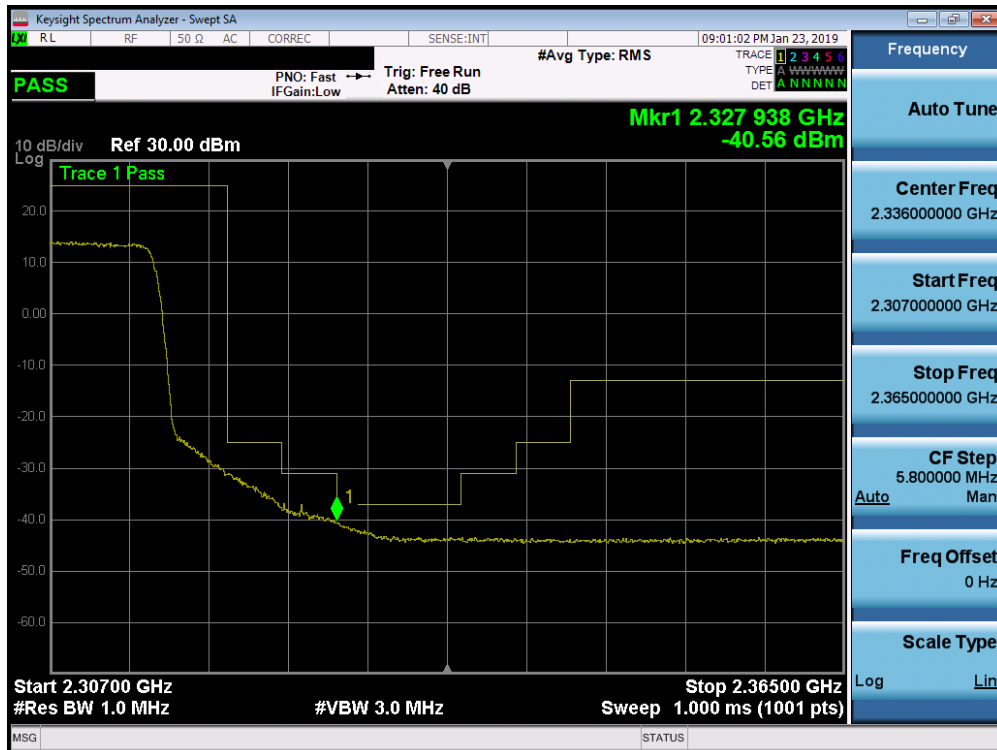
Plot 7-304. Upper Extended Band Edge Plot (Band 30 - 10.0MHz QPSK - Full RB Configuration)
