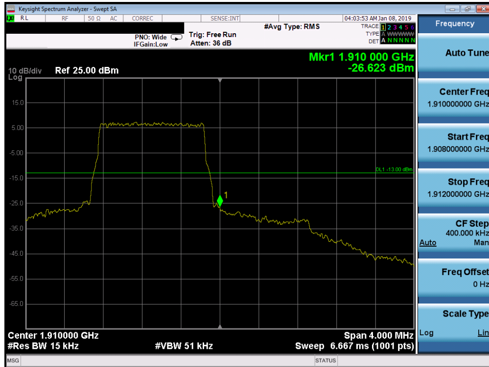
Plot 7-275. Upper Band Edge Plot (Band 2 - 1.4MHz QPSK - Full RB Configuration)
