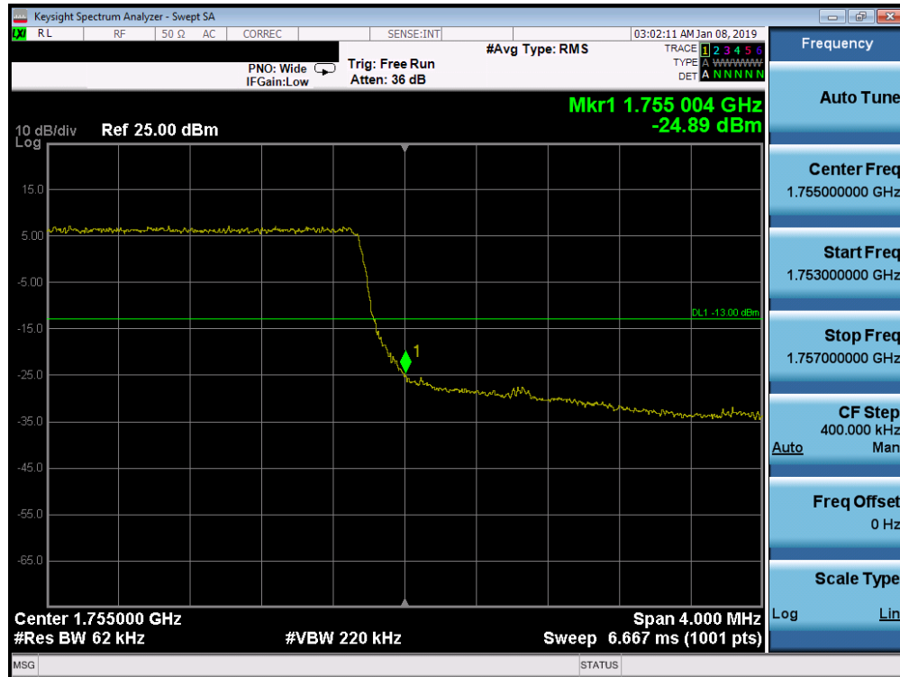
Plot 7-235. Upper Band Edge Plot (Band 4 - 5.0MHz QPSK - Full RB Configuration)
