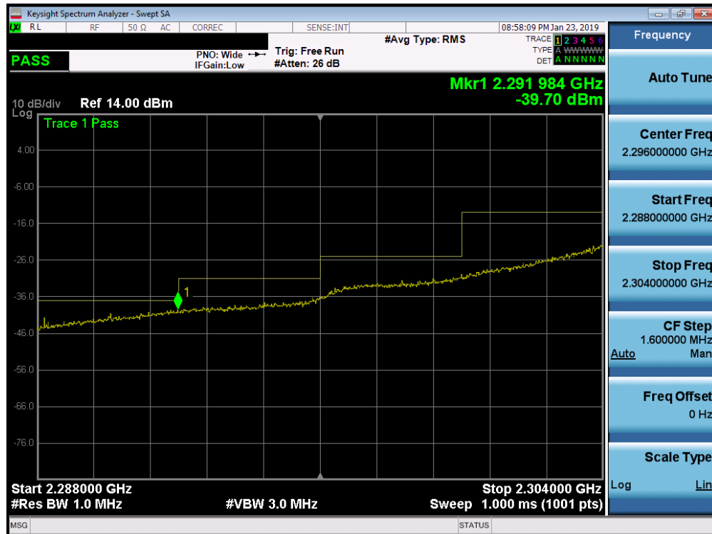
Plot 7-302. Lower Extended Band Edge Plot (Band 30 - 10.0MHz QPSK - Full RB Configuration)
