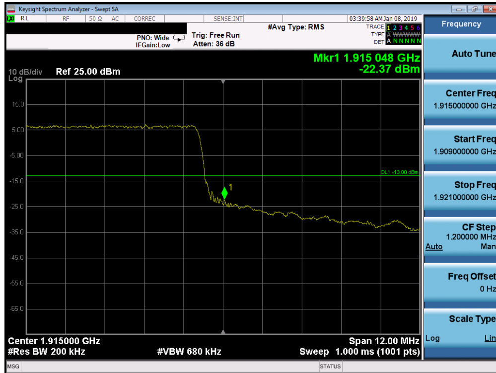
Plot 7-267. Upper Band Edge Plot (Band 25 - 15.0MHz QPSK - Full RB Configuration)
