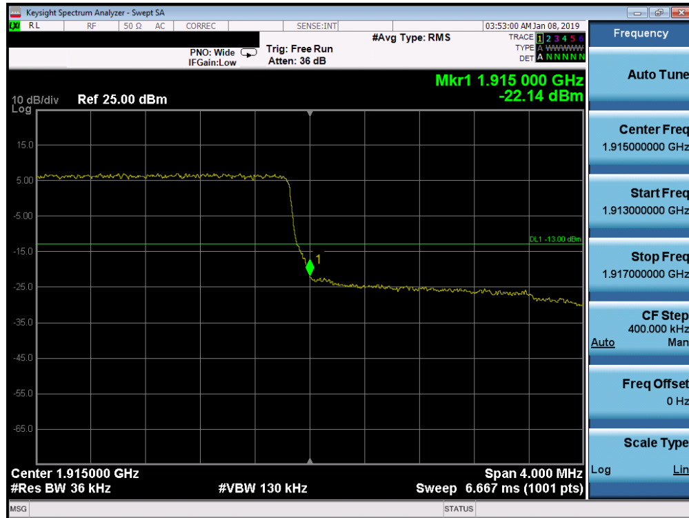
Plot 7-255. Upper Band Edge Plot (Band 25 - 3.0MHz QPSK - Full RB Configuration)
