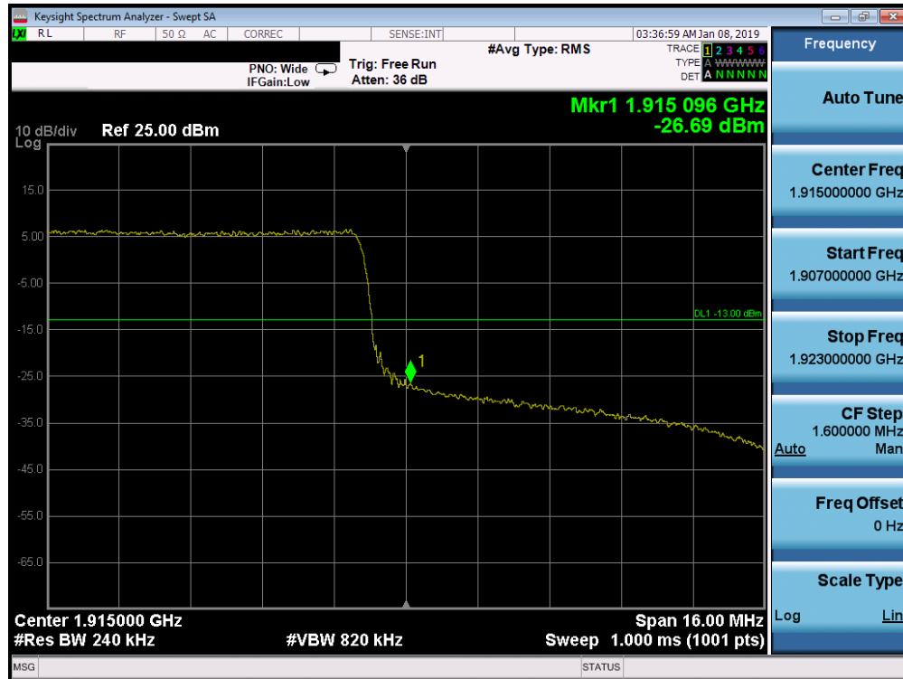
Plot 7-271. Upper Band Edge Plot (Band 25 - 20.0MHz QPSK - Full RB Configuration)
