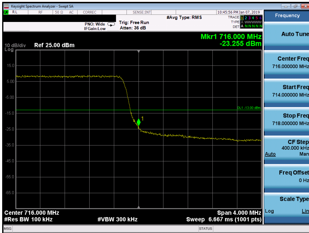
Plot 7-178. Upper Band Edge Plot (Band 17 - 5.0MHz QPSK - Full RB Configuration)
