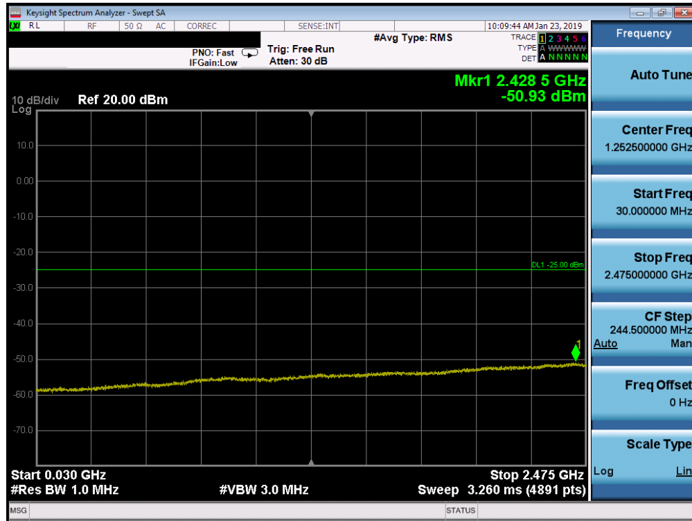
Plot 7-151. Conducted Spurious Plot (Band 7 - 20.0MHz QPSK - RB Size 1, RB Offset 0 - Low Channel)
