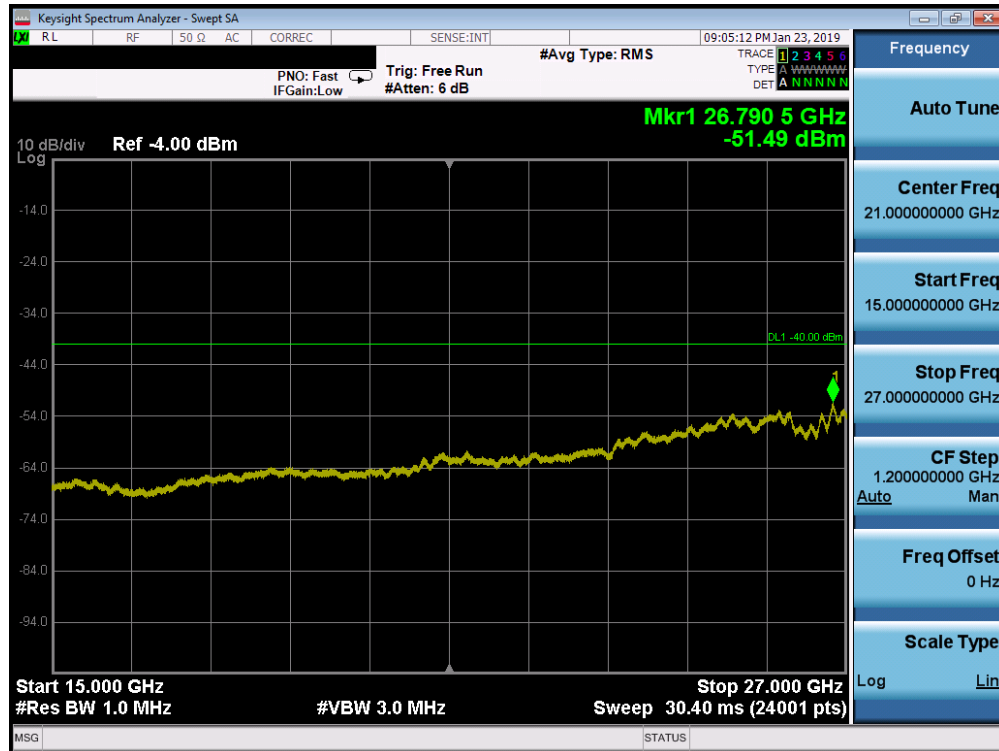
Plot 7-144. Conducted Spurious Plot (Band 30 - 10.0MHz QPSK - RB Size 1, RB Offset 0 - Low Channel)
