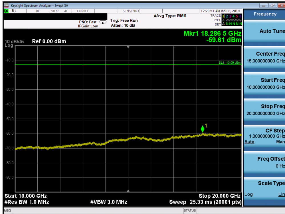
Plot 7-129. Conducted Spurious Plot (Band 66/4 - 20.0MHz QPSK - RB Size 1, RB Offset 0 - Mid Channel)
