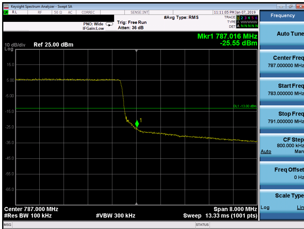
Plot 7-184. Upper Band Edge Plot (Band 13 -10.0MHz QPSK - Full RB Configuration)
