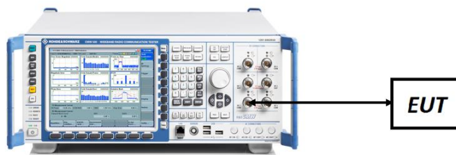
Figure 7-5. ERP/EIRP Measurement Setup
