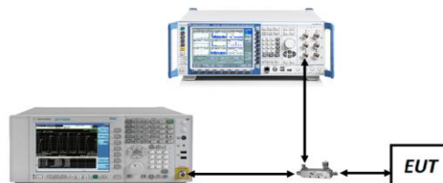
Figure 7-2. Test Instrument & Measurement Setup
