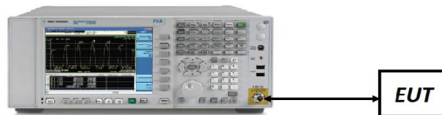
Figure 7-5. Test Instrument & Measurement Setup
