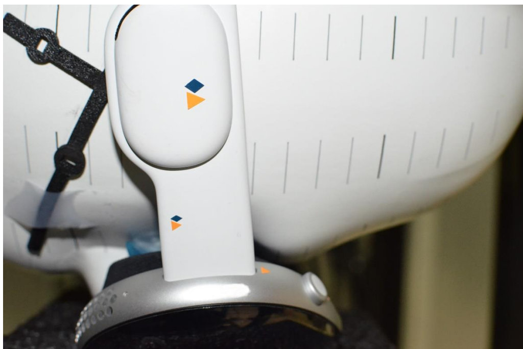
SAR Test Setup Photo 2: Antenna NB UNII-R Head SAR at 0.0 cm
