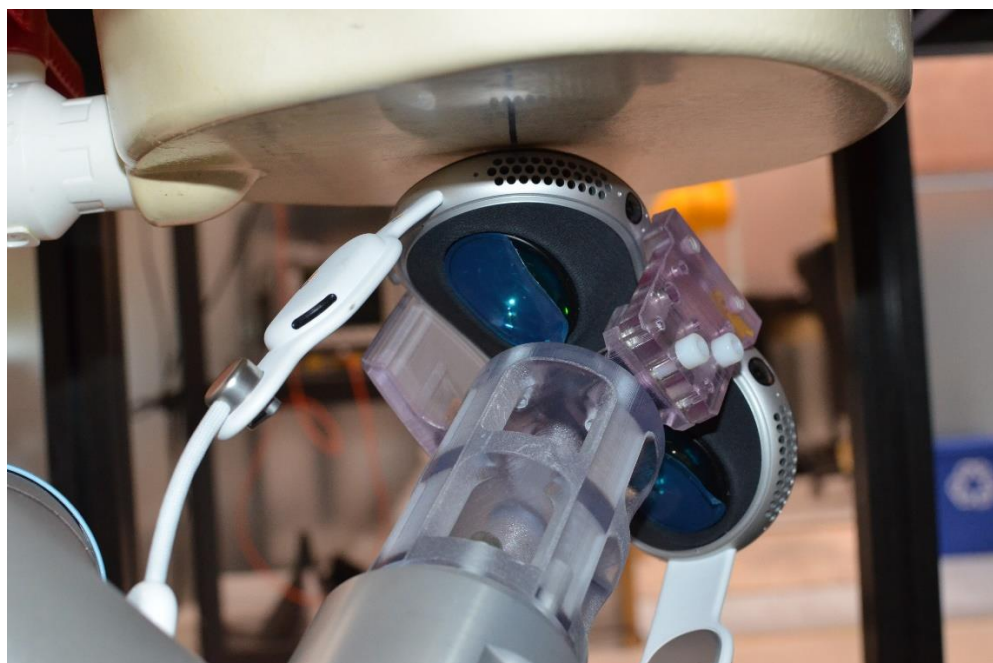
SAR Test Setup Photo 8: Antenna NB UNII_R Point 23 Extremity SAR at 0.0 cm
