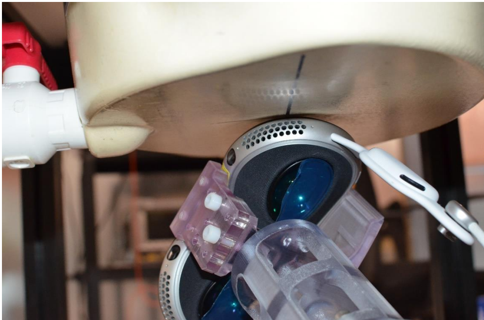
SAR Test Setup Photo 12: Antenna NB UNII_L Point 11 Extremity SAR at 0.0 cm
