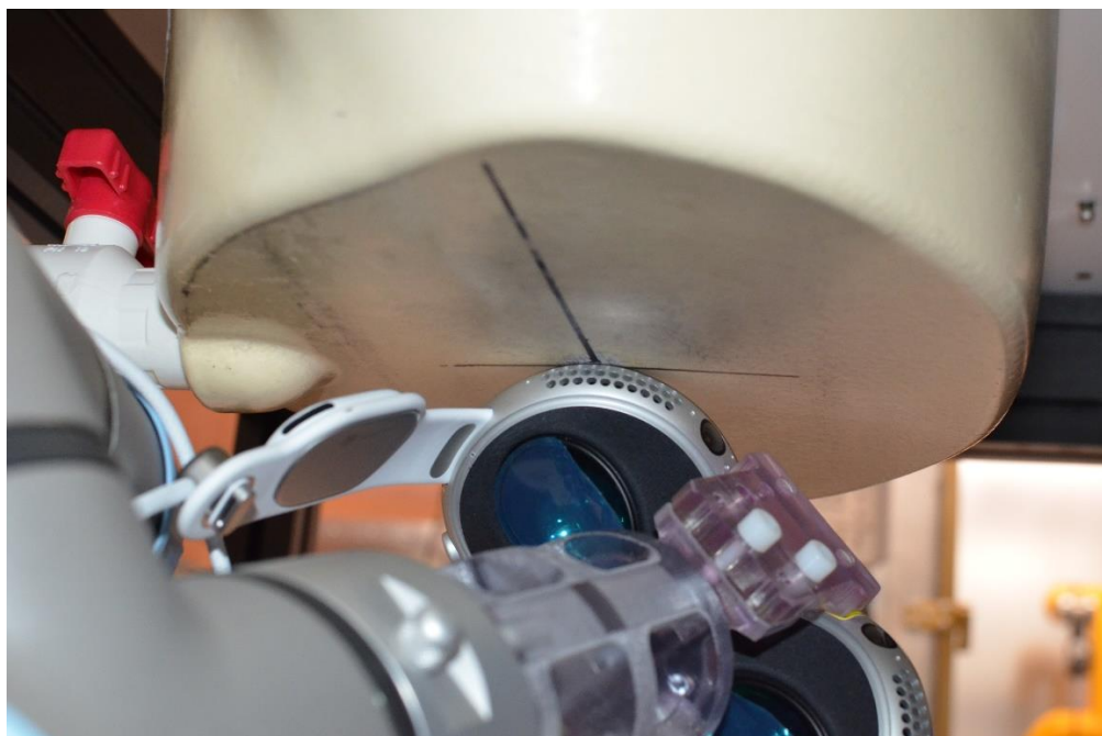
SAR Test Setup Photo 7: Antenna NB UNII_R Point 22 Extremity SAR at 0.0 cm
