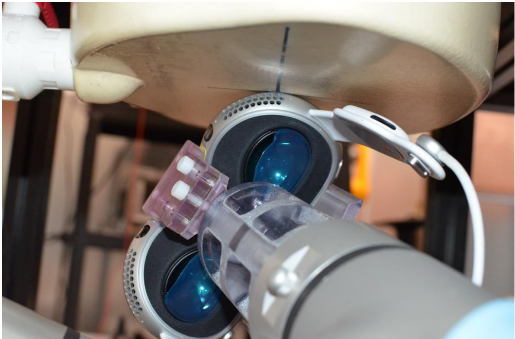
SAR Test Setup Photo 13: Antenna NB UNII_L Point 13 Extremity SAR at 0.0 cm
