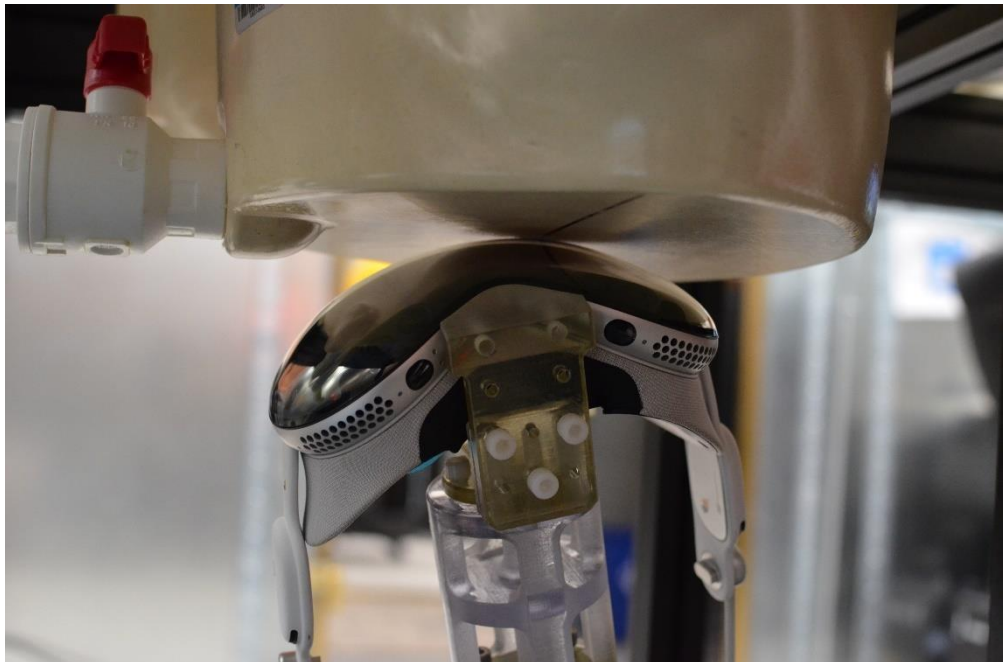
SAR Test Setup Photo 15: Antenna NB UNII_L Testing with Mini Light Seal Extremity SAR at 0.0 cm
