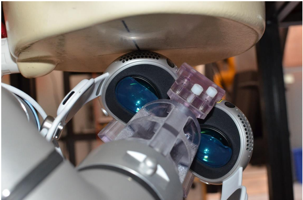
SAR Test Setup Photo 6: Antenna NB UNII_R Point 19 Extremity SAR at 0.0 cm
