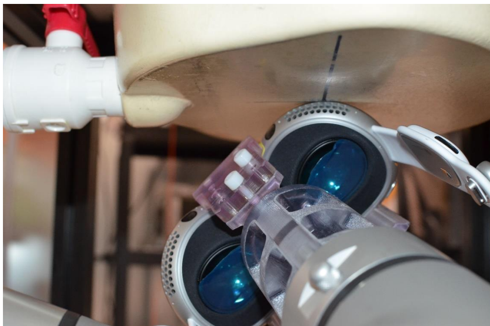
SAR Test Setup Photo 10: Antenna NB UNII_L Point 7 Extremity SAR at 0.0 cm
