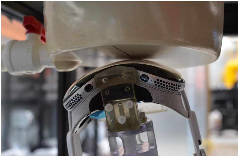
SAR Test Setup Photo 14: Antenna NB UNII_L Testing with Main Light Seal Extremity SAR at 0.0 cm
