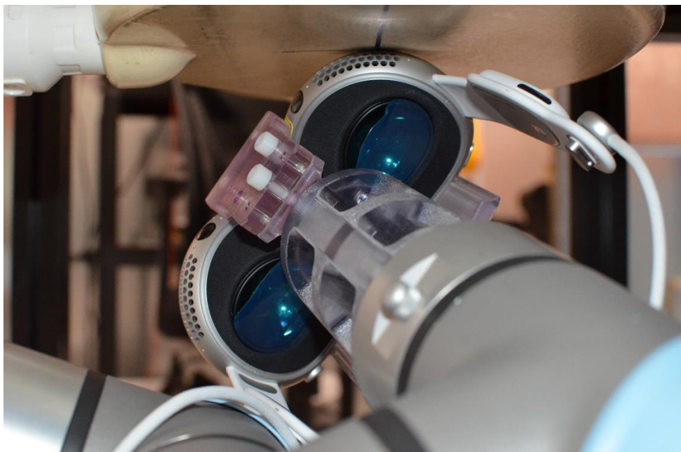
SAR Test Setup Photo 11: Antenna NB UNII_L Point 10 Extremity SAR at 0.0 cm
