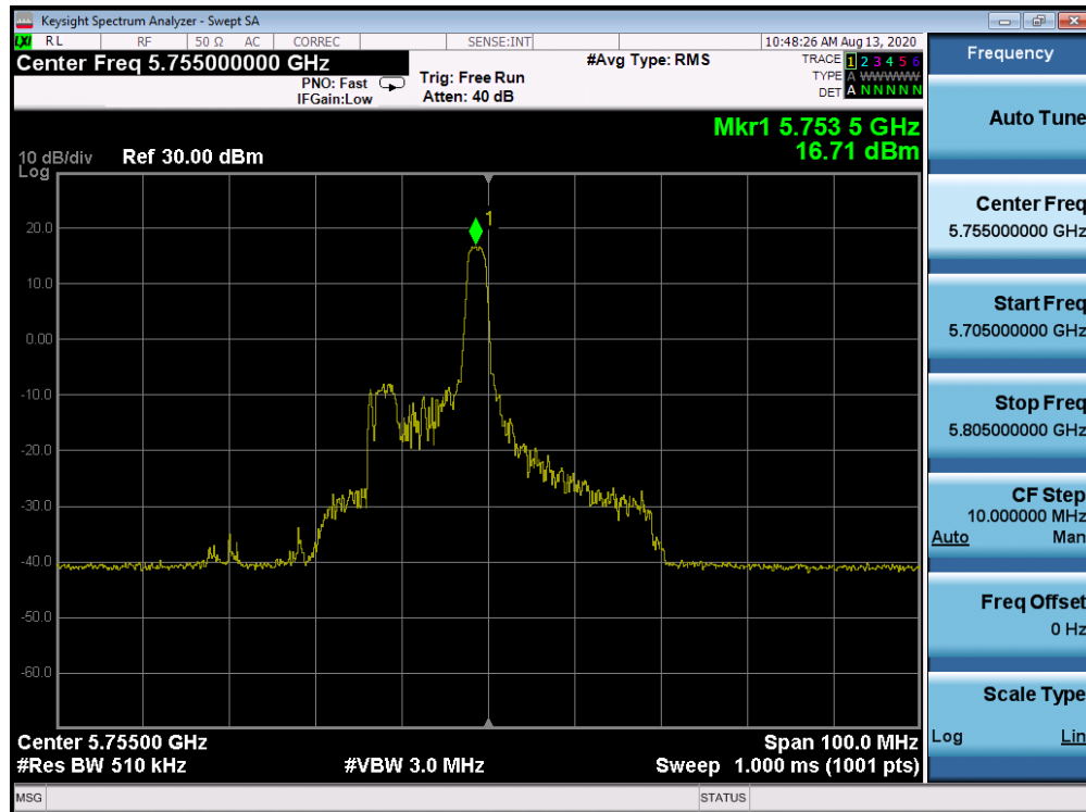
Plot 7-893. Power Spectral Density Plot CDD Primary Antenna 2b (40MHz BW 802.11ax Index 8 – RU26 (UNII Band 3) – Ch. 151)
