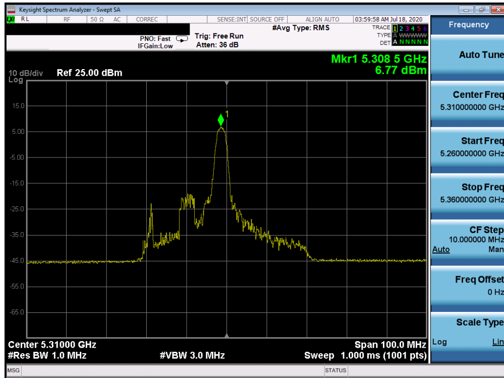
Plot 7-1043. Power Spectral Density Plot CDD Diversity Antenna 2b (40MHz BW 802.11ax Index 8 – RU26 (UNII Band 2A) – Ch. 62)
