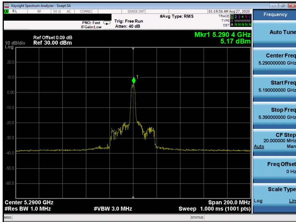
Plot 7-1053. Power Spectral Density Plot CDD Diversity Antenna 2b (80MHz BW 802.11ax Index 18 – RU26 (UNII Band 2A) – Ch. 58)
