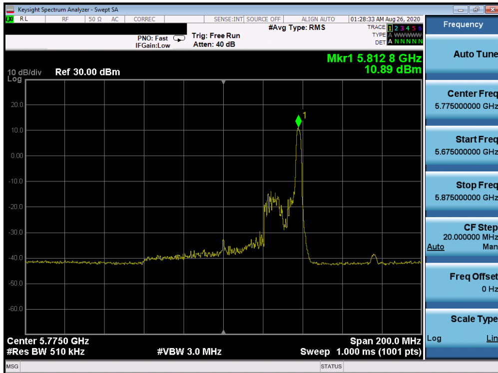
Plot 7-677. Power Spectral Density Plot Antenna 1b (80MHz BW 802.11ax Index 36 – RU26 (UNII Band 3) – Ch. 155)
