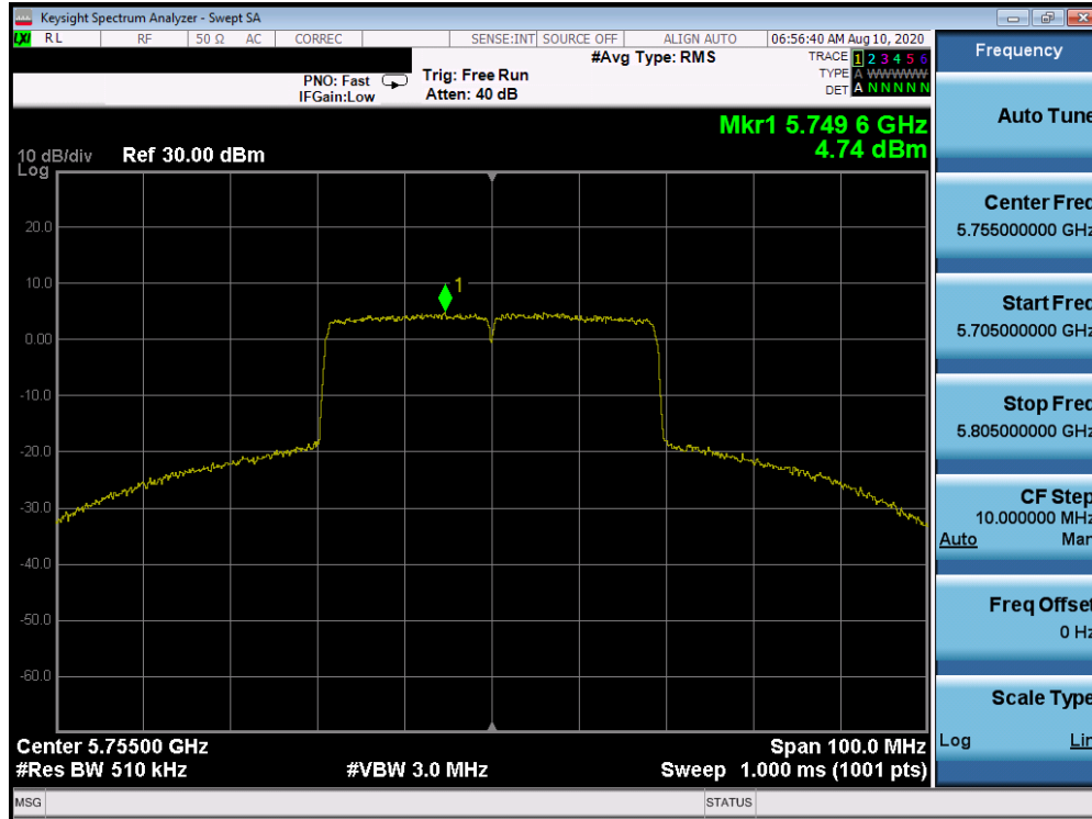
Plot 7-673. Power Spectral Density Plot Antenna 1b (40MHz BW 802.11ax – RU484 (UNII Band 3) – Ch. 151)
