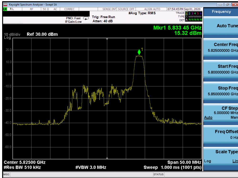
Plot 7-663. Power Spectral Density Plot Antenna 1b (20MHz BW 802.11ax Index 8 – RU26 (UNII Band 3) – Ch. 165)
