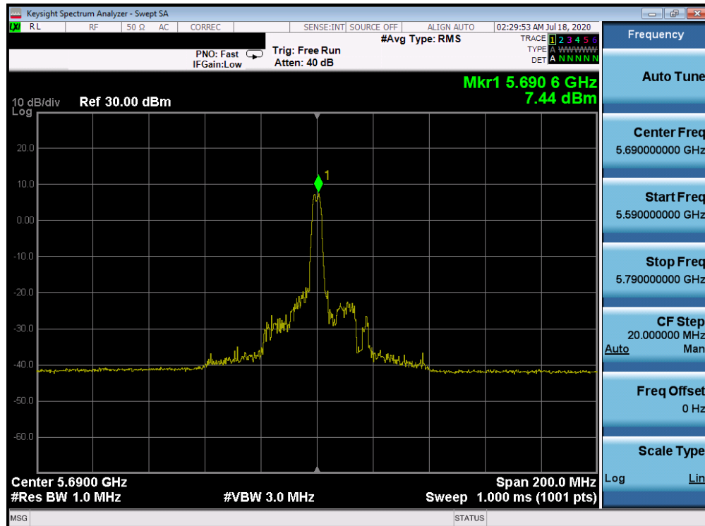
Plot 7-650. Power Spectral Density Plot Antenna 1b (80MHz BW 802.11ax Index 18 – RU26 (UNII Band 2C) – Ch. 138)
