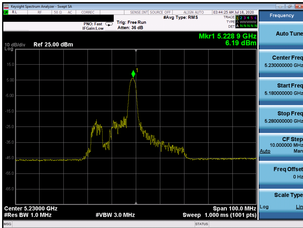
Plot 7-735. Power Spectral Density Plot CDD Primary Antenna 2b (40MHz BW 802.11ax Index 8 – RU26 (UNII Band 1) – Ch. 46)
