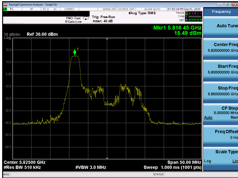
Plot 7-661. Power Spectral Density Plot Antenna 1b (20MHz BW 802.11ax Index 0 – RU26 (UNII Band 3) – Ch. 165)
