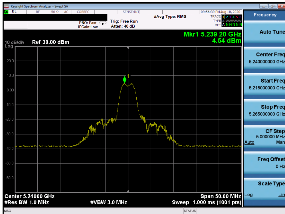
Plot 7-686. ISED Power Spectral Density Plot Antenna 1b (20MHz BW 802.11ax Index 4 – RU26 (UNII Band 1) – Ch. 48)
