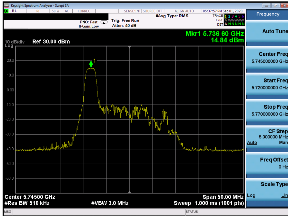
Plot 7-655. Power Spectral Density Plot Antenna 1b (20MHz BW 802.11ax Index 0 – RU26 (UNII Band 3) – Ch. 149)
