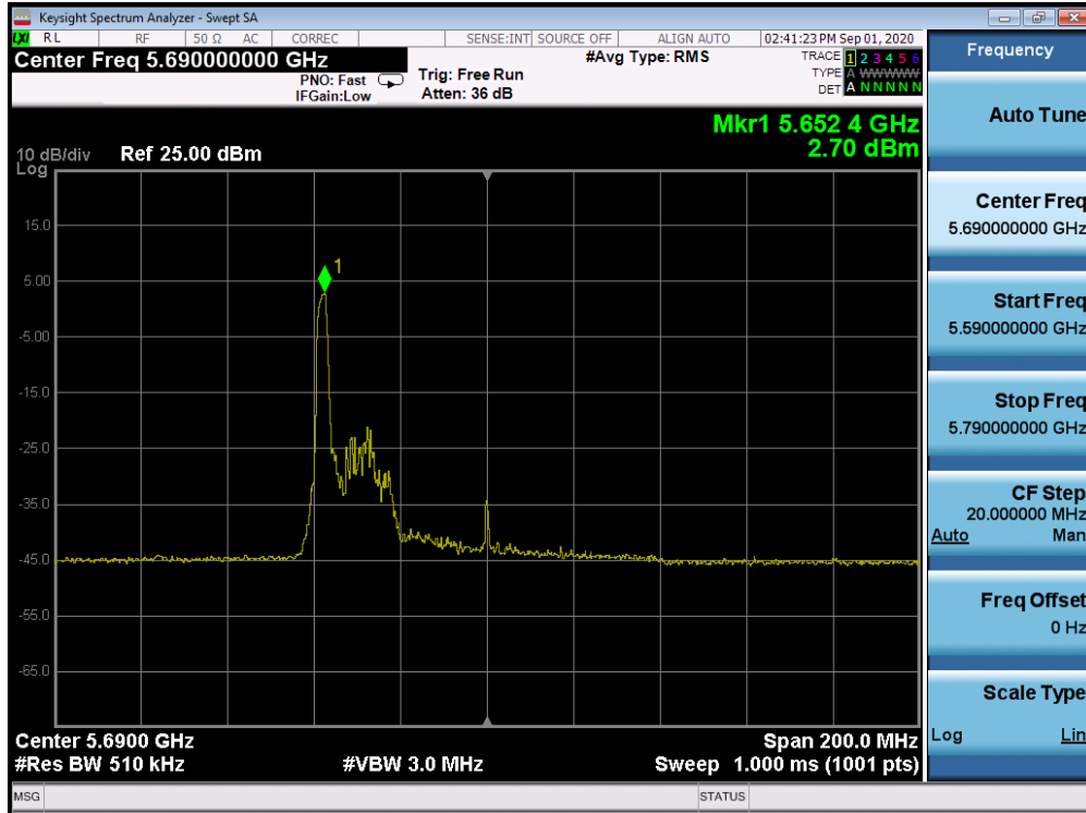
Plot 7-519. Power Spectral Density Plot Antenna 2a (80MHz BW 802.11ax Index 0 – RU26 (UNII Band 2C) – Ch. 138)
