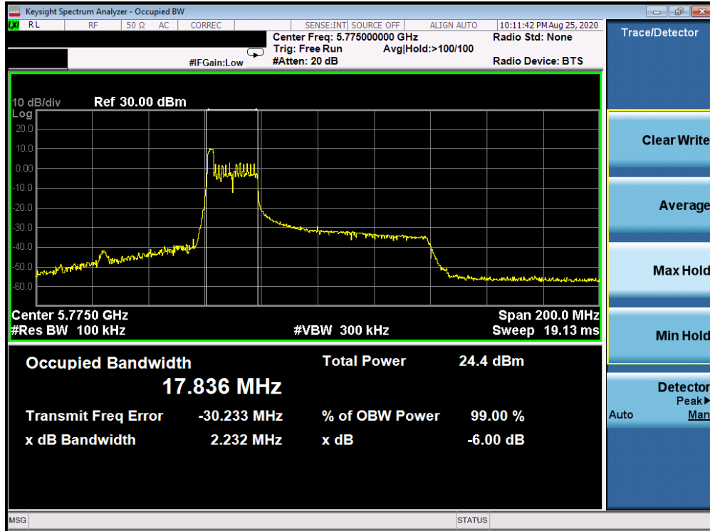
Plot 7-285. 6dB Bandwidth Plot Antenna 2a (80MHz BW 802.11ax Index 0 – RU26 (UNII Band 3) – Ch. 155)
