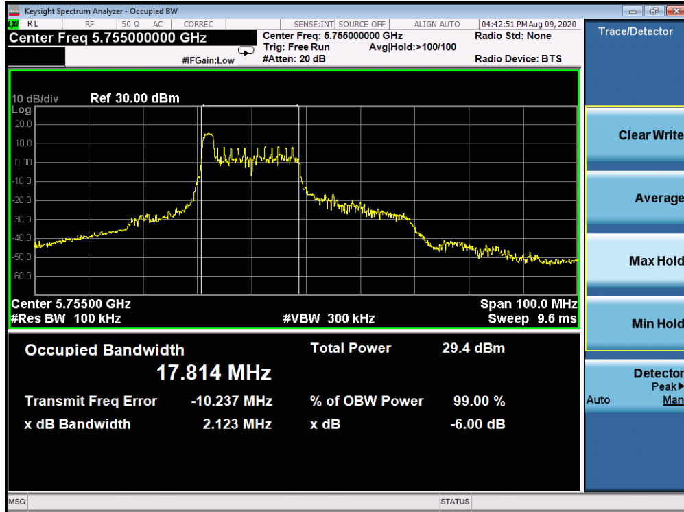
Plot 7-301. 6dB Bandwidth Plot Antenna 1b (40MHz BW 802.11ax Index 0 – RU26 (UNII Band 3) – Ch. 151)
