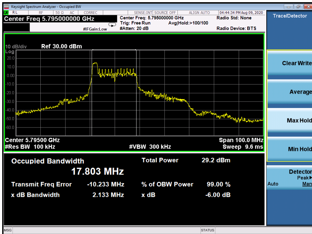
Plot 7-304. 6dB Bandwidth Plot Antenna 1b (40MHz BW 802.11ax Index 0 – RU26 (UNII Band 3) – Ch. 159)
