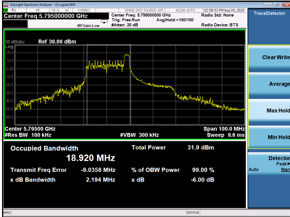
Plot 7-257. 6dB Bandwidth Plot Antenna 2b (40MHz BW 802.11ax Index 8 – RU26 (UNII Band 3) – Ch. 159)
