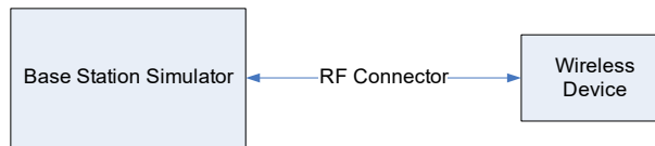
Figure 8-2 Power Measurement Setup
