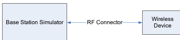
Figure 8-1 Power Measurement Setup
