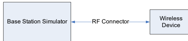
Figure 8-3 Power Measurement Setup
