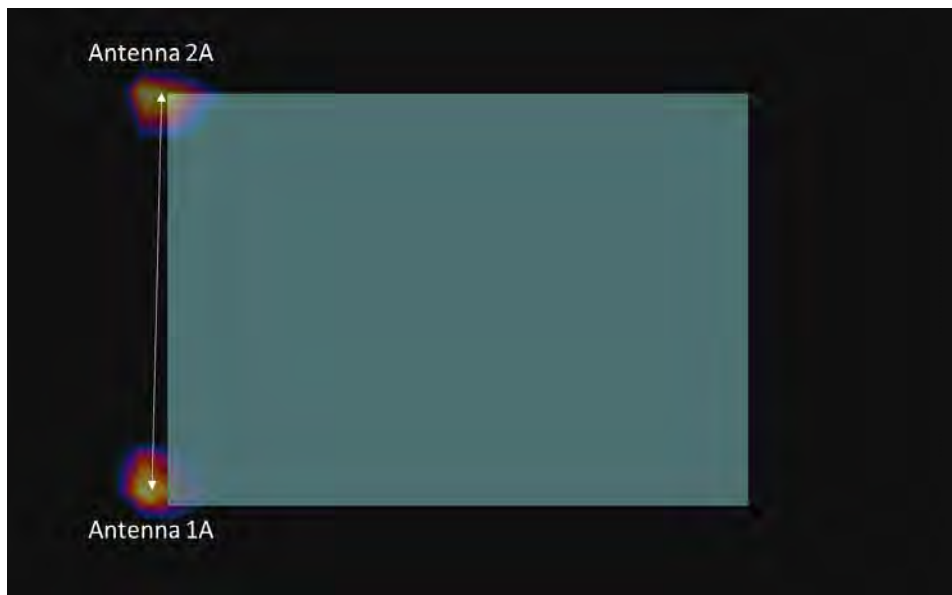
Figure 11-11 Back Side Spatial Separation for Antenna 1A and Antenna 2A
