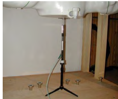
Figure 9-2 System Verification Setup Photo
