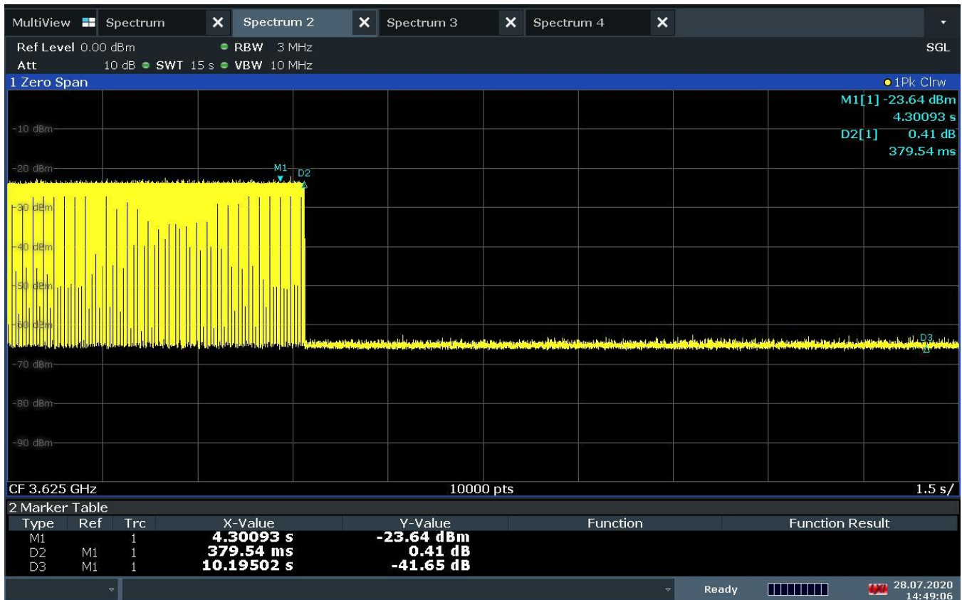
Plot 7-37. Run#1 End User Device Discontinues Operations within 10s
