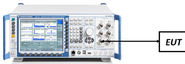
Figure 7-4. ERP/EIRP Measurement Setup
