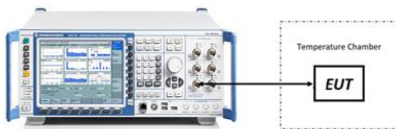
Figure 7-6. Test Instrument & Measurement Setup
