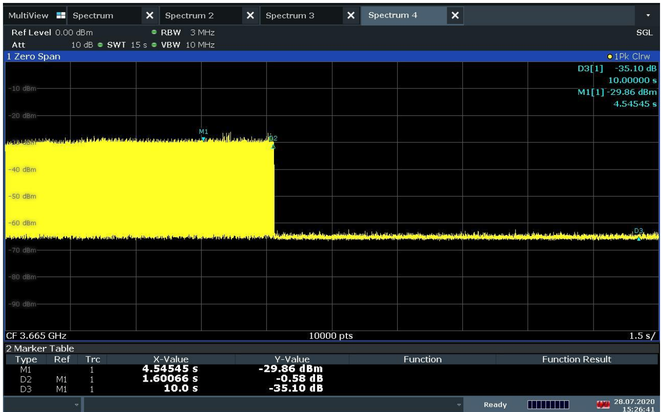
Plot 7-39. Run#2 End User Device Discontinues Operations within 10s
