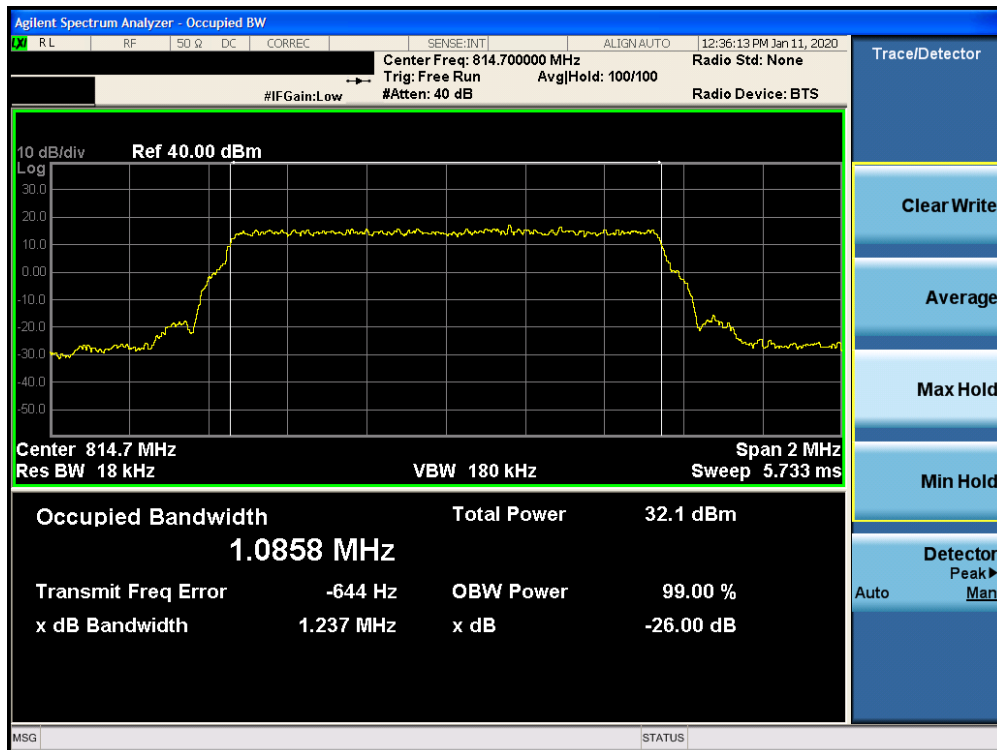
Plot 7-12. Occupied Bandwidth Plot (LTE Band 26 - 1.4MHz 64-QAM - Full RB Configuration)
