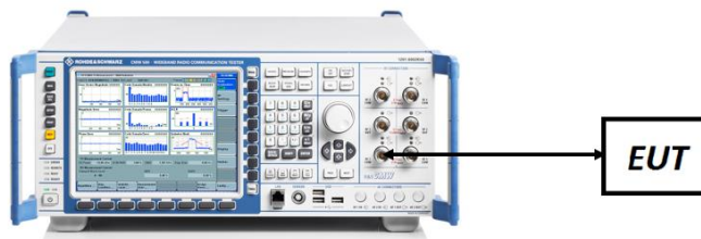
Figure 7-4. Conducted Power Measurement Setup
