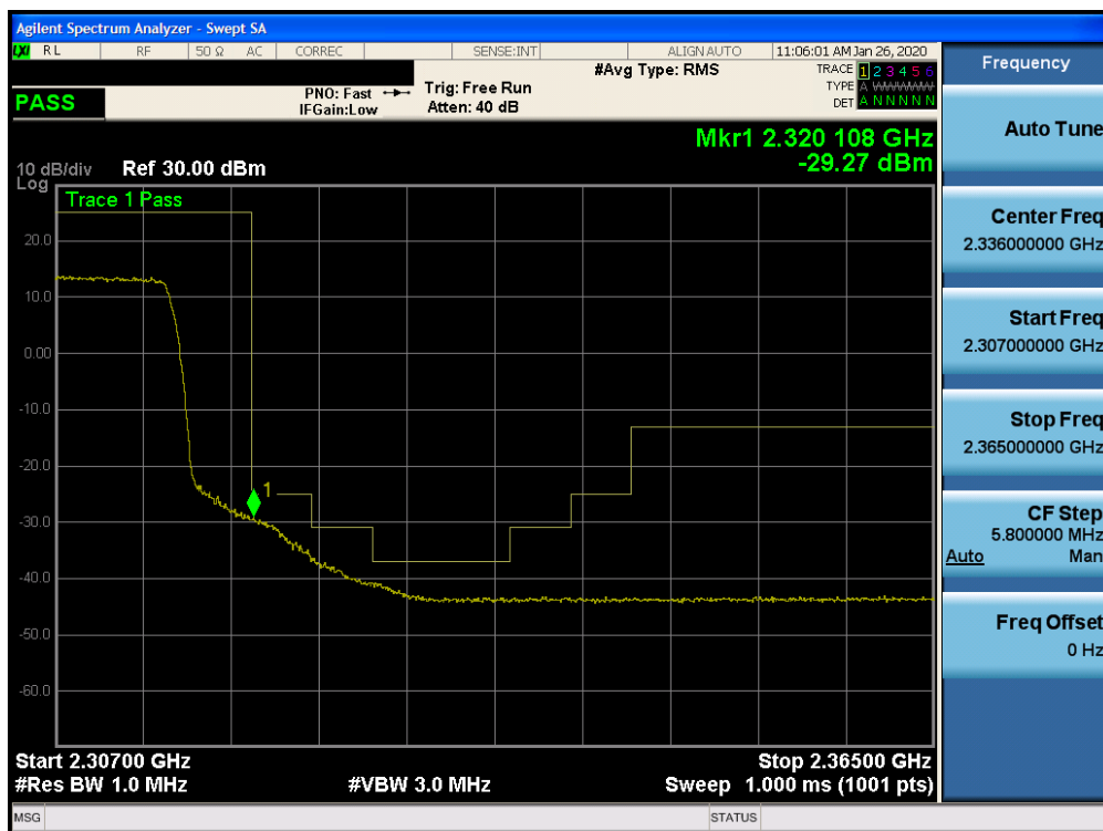
Plot 7-337. Upper Extended Band Edge Plot (Band 30 – 10.0MHz QPSK – RB Size 50)
