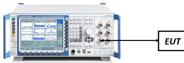
Figure 7-5. ERP/EIRP Measurement Setup
