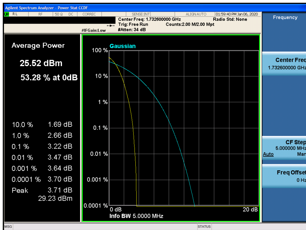
Plot 7-74. Peak-Average Ratio Plot (AWS WCDMA Mode)
