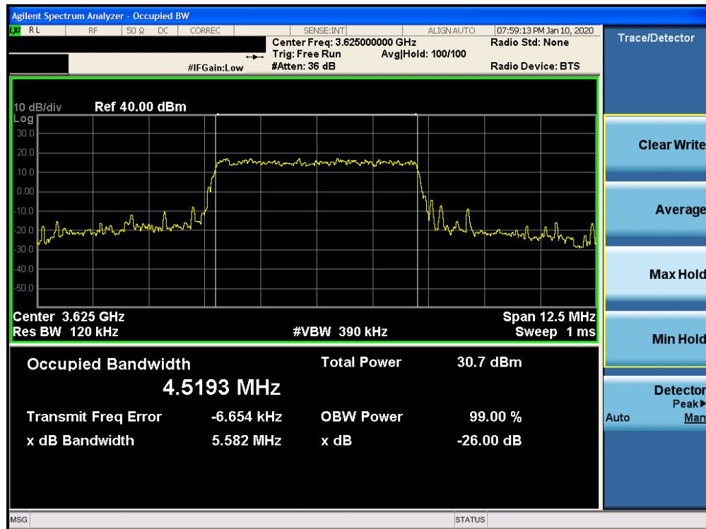
Plot 7-11. Occupied Bandwidth Plot (LTE Band 48 - 5MHz 16-QAM - Full RB Configuration)
