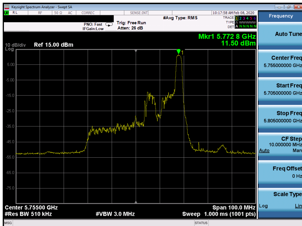
Plot 7-702. Power Spectral Density Plot CDD CORE 1 (40MHz BW 802.11ax Index 17 – RU26 (UNII Band 3) – Ch. 151)
