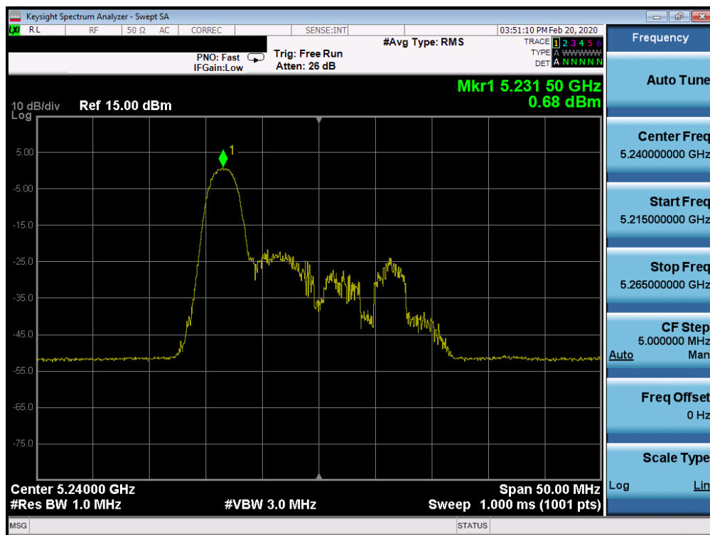
Plot 7-638. Power Spectral Density Plot ISED CDD CORE 1 (20MHz BW 802.11ax Index 0 – RU26 (UNII Band 1) – Ch. 48)
