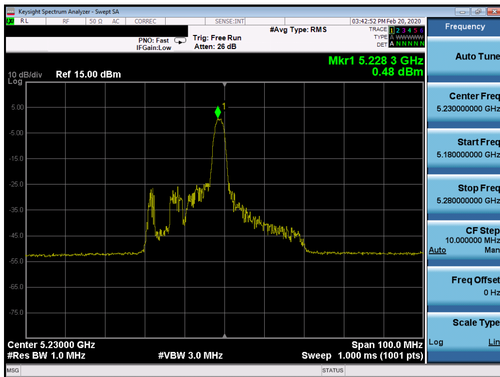
Plot 7-658. Power Spectral Density Plot ISED CDD CORE 1 (40MHz BW 802.11ax Index 8 – RU26 (UNII Band 1) – Ch. 46)
