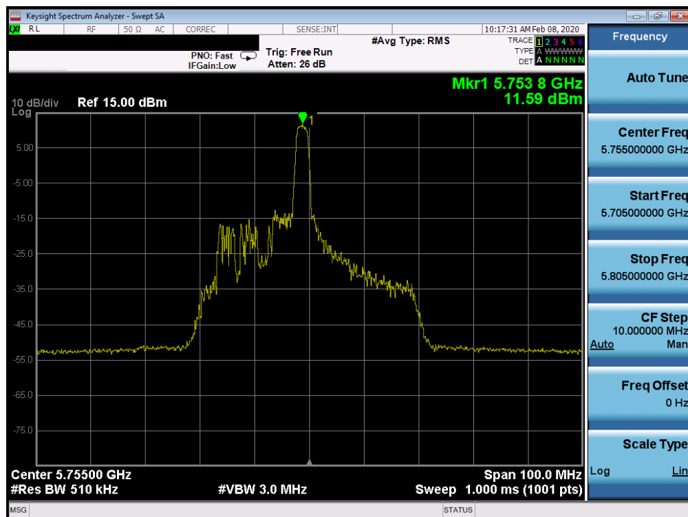
Plot 7-700. Power Spectral Density Plot CDD CORE 1 (40MHz BW 802.11ax Index 8 – RU26 (UNII Band 3) – Ch. 151)
