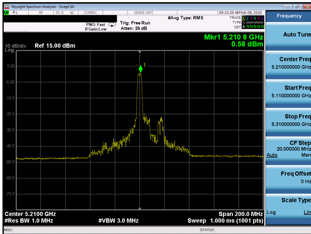
Plot 7-668. Power Spectral Density Plot ISED CDD CORE 1 (80MHz BW 802.11ax Index 18 – RU26 (UNII Band 1) – Ch. 42)
