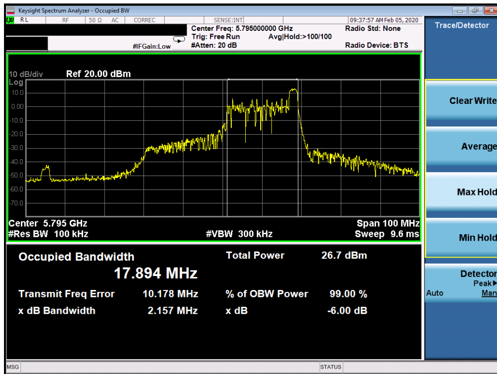
Plot 7-178. 6dB Bandwidth Plot SISO CORE 0 (40MHz BW 802.11ax Index 17 – RU26 (UNII Band 3) – Ch. 159)
