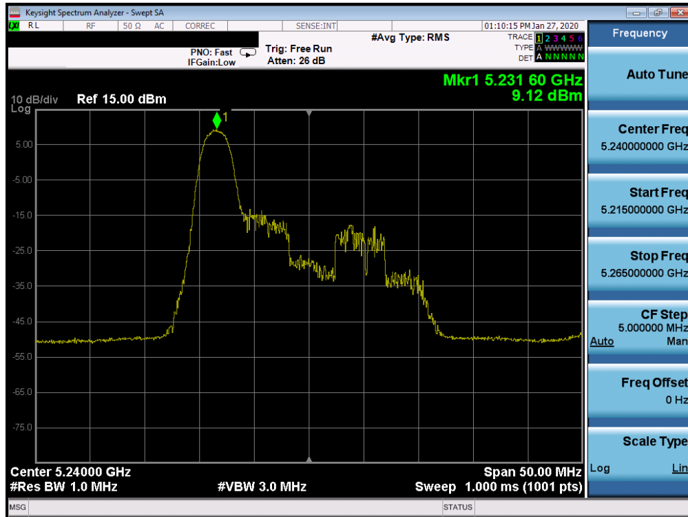
Plot 7-215. Power Spectral Density Plot SISO CORE 0 (20MHz BW 802.11ax Index 0 – RU26 (UNII Band 1) – Ch. 48)
