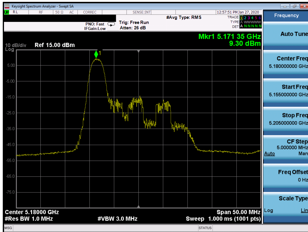
Plot 7-209. Power Spectral Density Plot SISO CORE 0 (20MHz BW 802.11ax Index 0 – RU26 (UNII Band 1) – Ch. 36)
