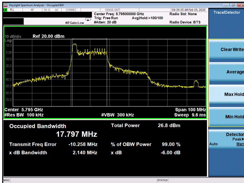
Plot 7-176. 6dB Bandwidth Plot SISO CORE 0 (40MHz BW 802.11ax Index 0 – RU26 (UNII Band 3) – Ch. 159)
