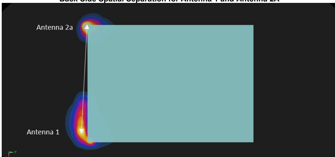
Figure 11-1 Back Side Spatial Separation for Antenna 1 and Antenna 2A
