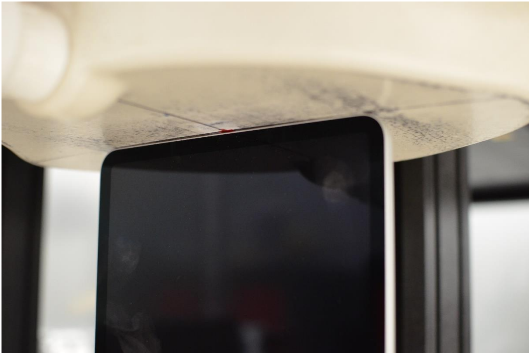
SAR Test Setup Photo 4: Bottom Edge at 0.0 cm
