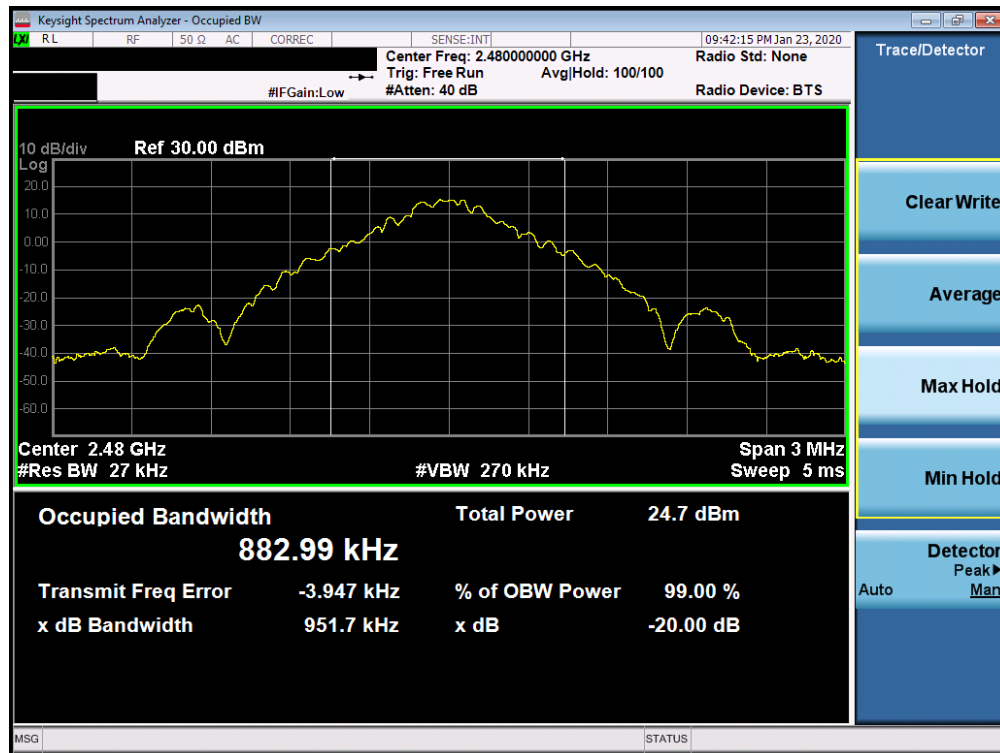
Plot 7-9. 20dB Bandwidth Plot Ant 2a (Bluetooth, GFSK, ePA – Ch. 78)
