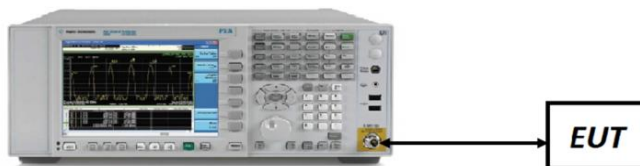
Figure 7-3. Test Instrument & Measurement Setup
