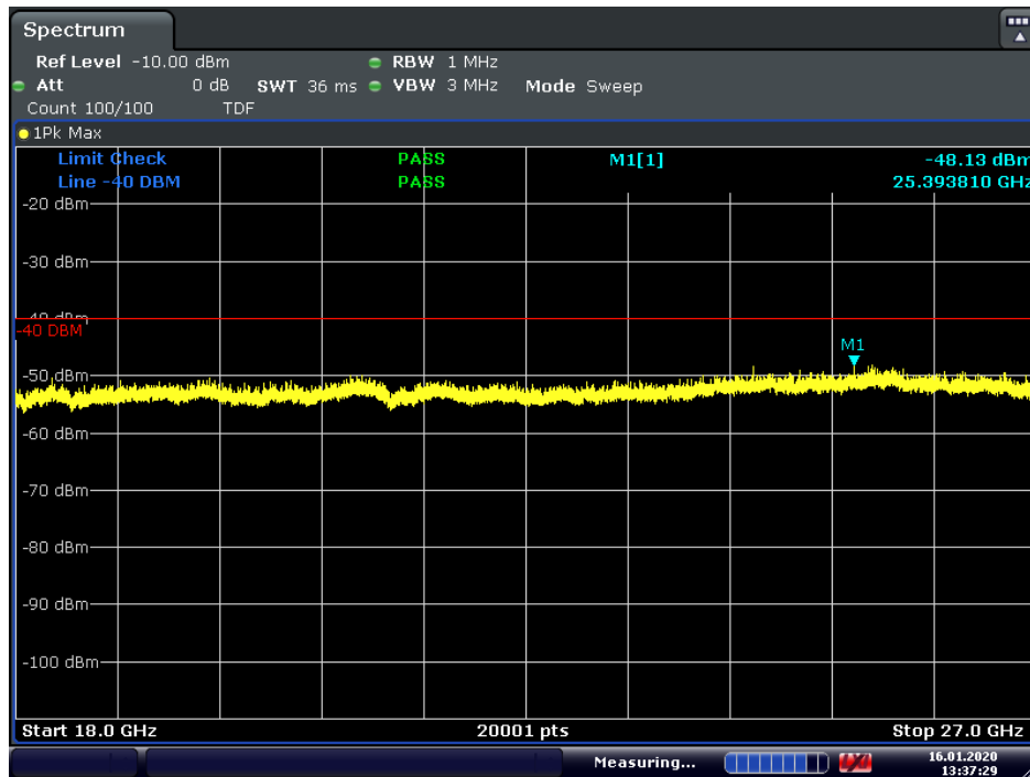
Plot 7-460. Radiated Spurious Plot 18GHz – 27GHz V (Band 30)
