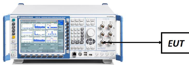
Figure 7-5. Conducted Power Measurement Setup
