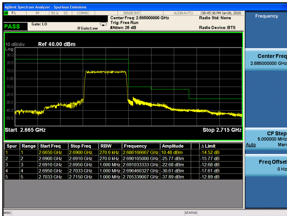
Plot 7-349. Upper ACP Plot (Band 41 – 10.0MHz QPSK – RB Size 50)
