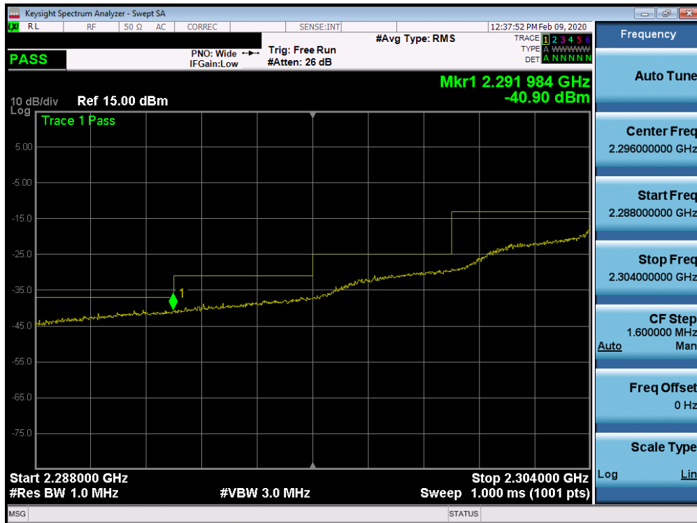
Plot 7-331. Lower Extended Band Edge Plot (Band 30 – 5.0MHz QPSK – RB Size 25)
