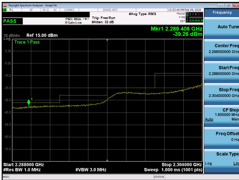
Plot 7-335. Lower Extended Band Edge Plot (Band 30 – 10.0MHz QPSK – RB Size 50)
