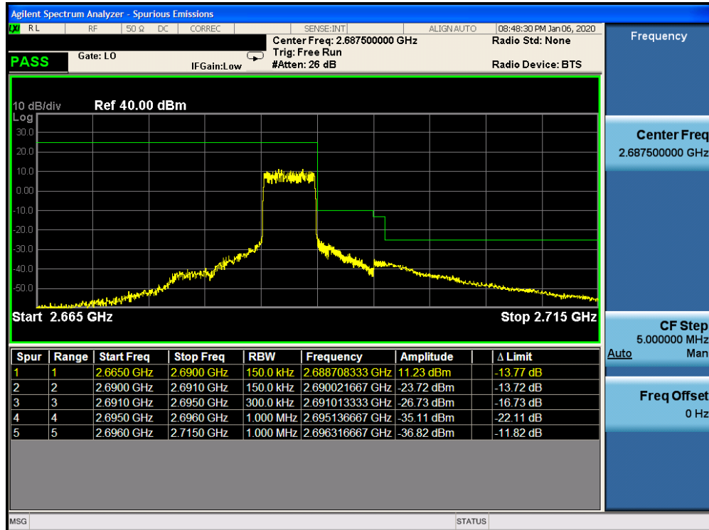
Plot 7-347. Upper ACP Plot (Band 41 – 5.0MHz QPSK – RB Size 25)
