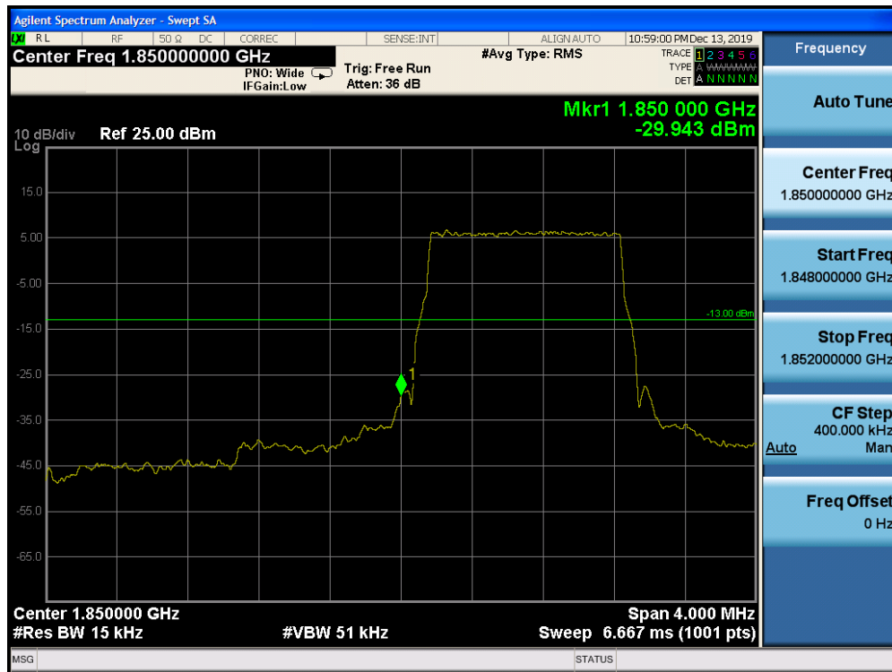
Plot 7-306. Lower Band Edge Plot (Band 25 – 1.4MHz QPSK – RB Size 6)
