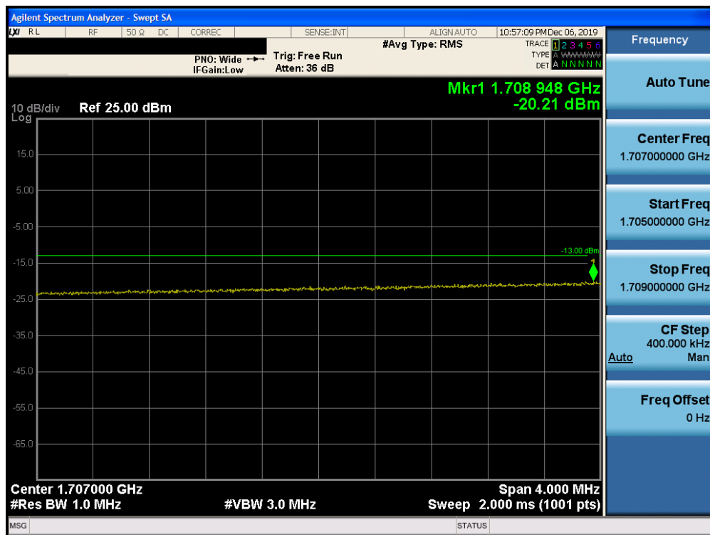
Plot 7-255. Lower Extended Band Edge Plot (Band 4 – 20.0MHz QPSK – RB Size 100)
