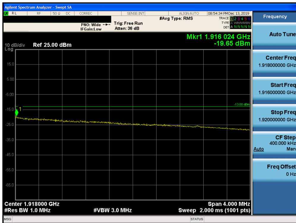
Plot 7-321. Upper Extended Band Edge Plot (Band 25 – 10.0MHz QPSK – RB Size 50)
