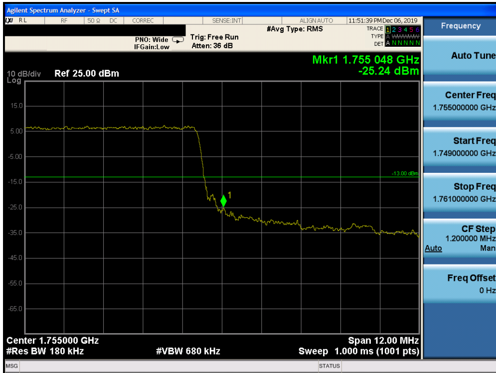
Plot 7-252. Upper Band Edge Plot (Band 4 – 15.0MHz QPSK – RB Size 75)
