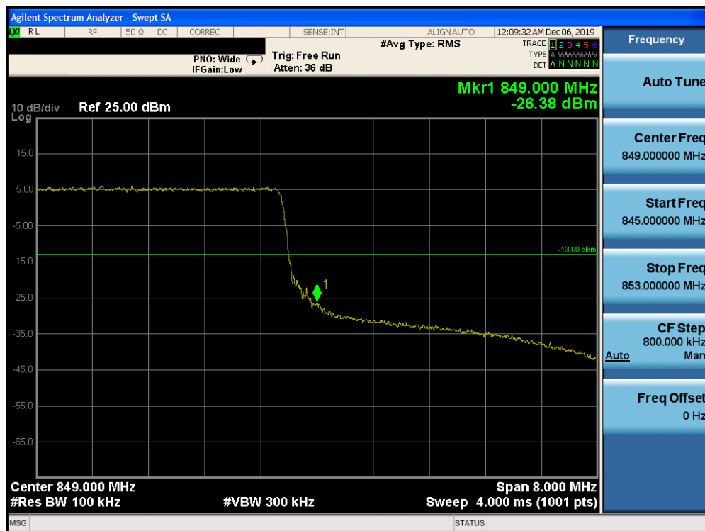
Plot 7-233. Upper Band Edge Plot (Band 5 - 10.0MHz QPSK - RB Size 50)
