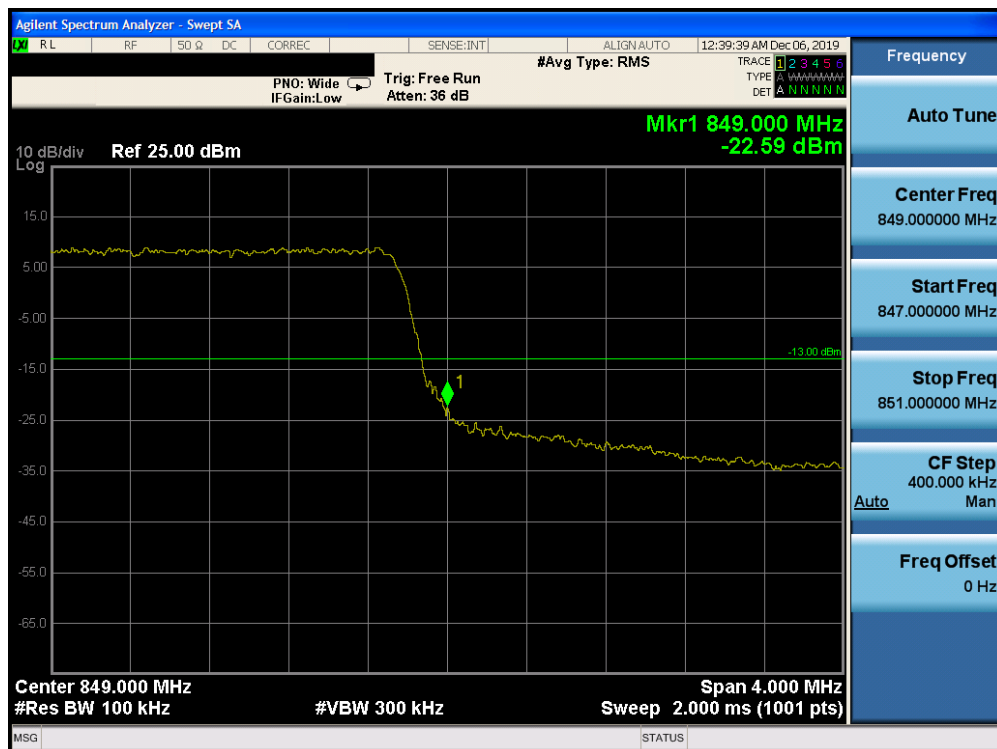
Plot 7-231. Upper Band Edge Plot (Band 5 – 5.0MHz QPSK – RB Size 25)
