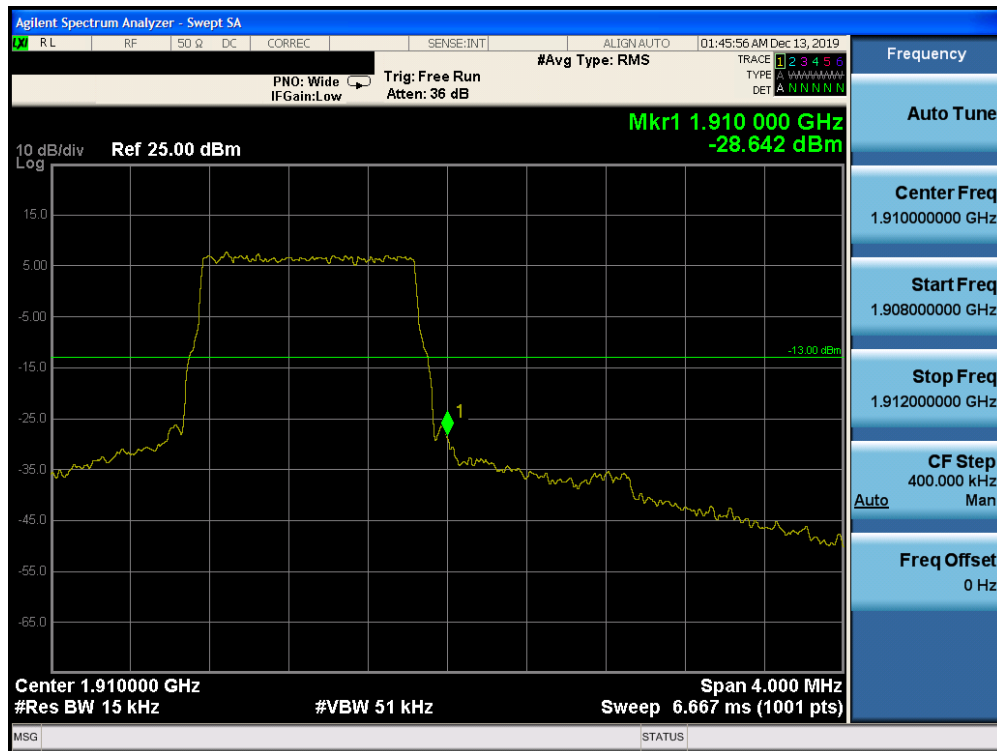
Plot 7-284. Upper Band Edge Plot (Band 2 – 1.4MHz QPSK – RB Size 6)
