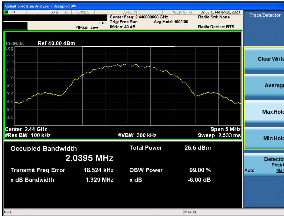
Plot 7-11. 6dB Bandwidth Plot Ant 2a (Bluetooth (LE), 2Mbps, ePA – Ch. 19)
