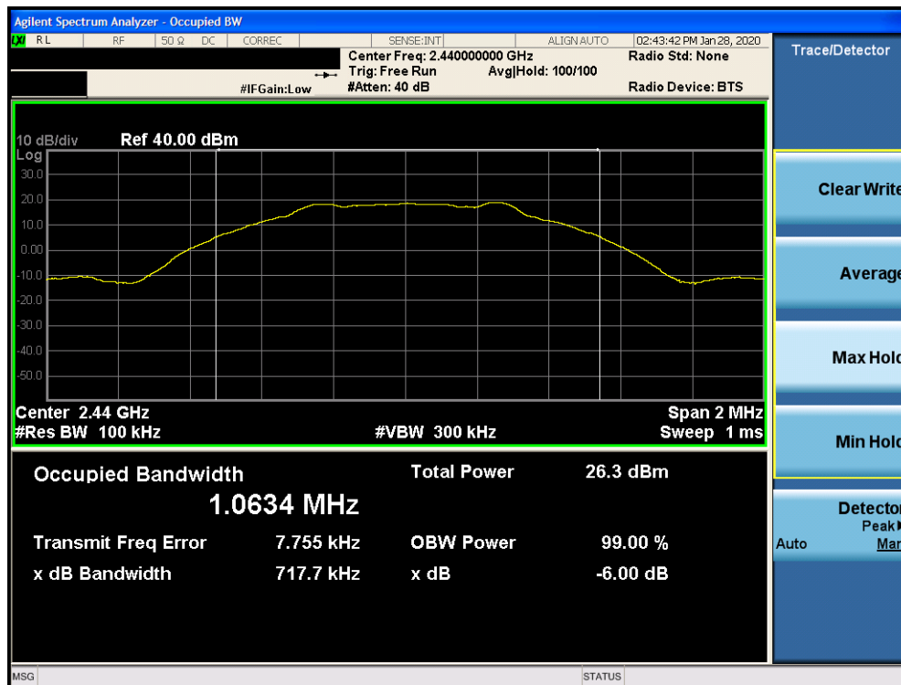
Plot 7-8. 6dB Bandwidth Plot Ant 2a (Bluetooth (LE), 1Mbps, ePA – Ch. 19)
