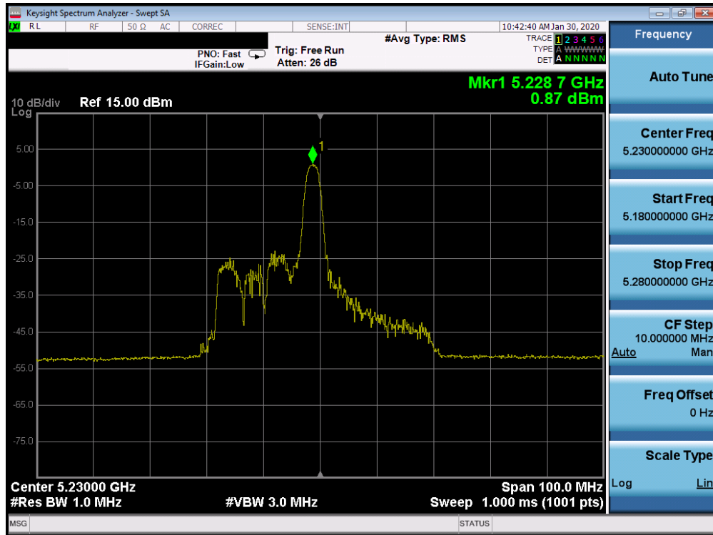
Plot 7-657. Power Spectral Density Plot ISED CDD CORE 0 (40MHz BW 802.11ax Index 8 – RU26 (UNII Band 1) – Ch. 46)
