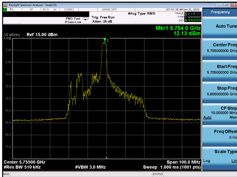
Plot 7-699. Power Spectral Density Plot CDD CORE 0 (40MHz BW 802.11ax Index 8 – RU26 (UNII Band 3) – Ch. 151)
