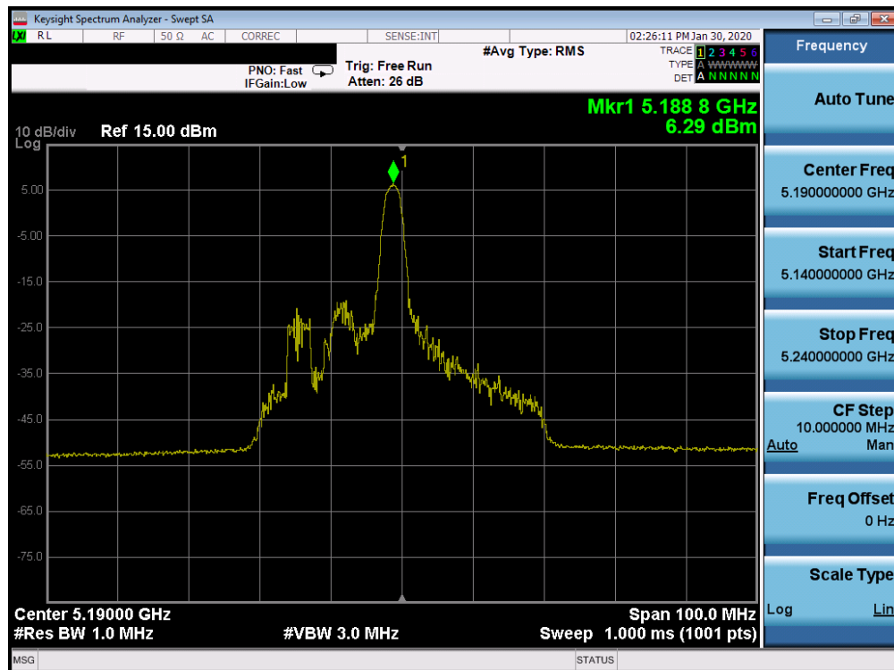
Plot 7-492. Power Spectral Density Plot CDD CORE 1 (40MHz BW 802.11ax Index 8 – RU26 (UNII Band 1) – Ch. 38)
