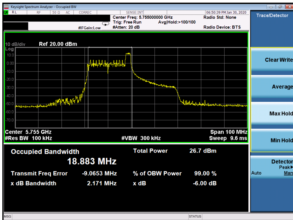
Plot 7-198. 6dB Bandwidth Plot SISO CORE 1 (40MHz BW 802.11ax Index 8 – RU26 (UNII Band 3) – Ch. 151)
