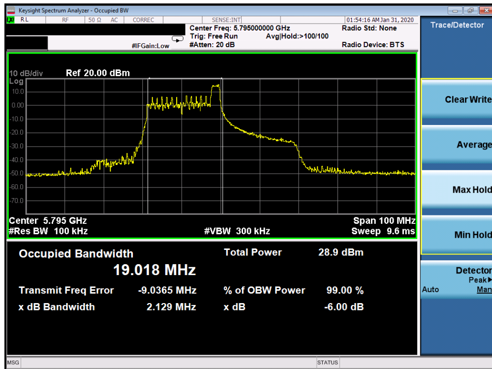
Plot 7-177. 6dB Bandwidth Plot SISO CORE 0 (40MHz BW 802.11ax Index 8 – RU26 (UNII Band 3) – Ch. 159)
