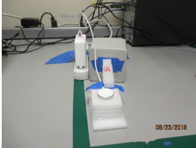
S1, RF EXPOSURE SETUP PHOTO @ 15 cm
