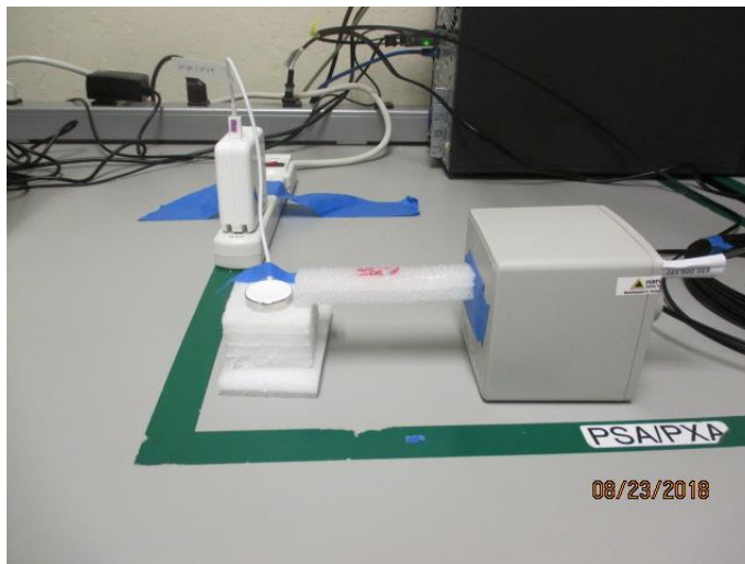
S2, RF EXPOSURE SETUP PHOTO @ 15 cm
