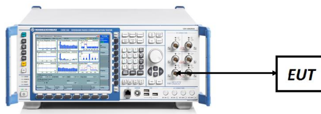
Figure 7-6. ERP/EIRP Measurement Setup
