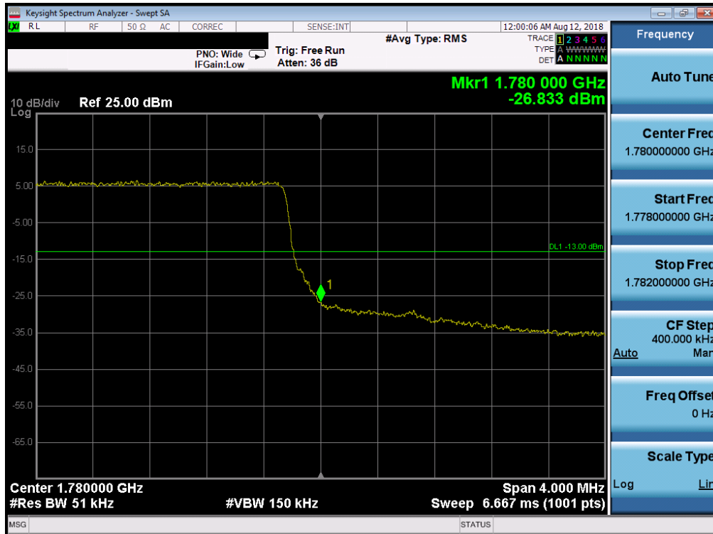
Plot 7-256. Upper Band Edge Plot (Band 66 – 5.0MHz QPSK – RB Size 25)
