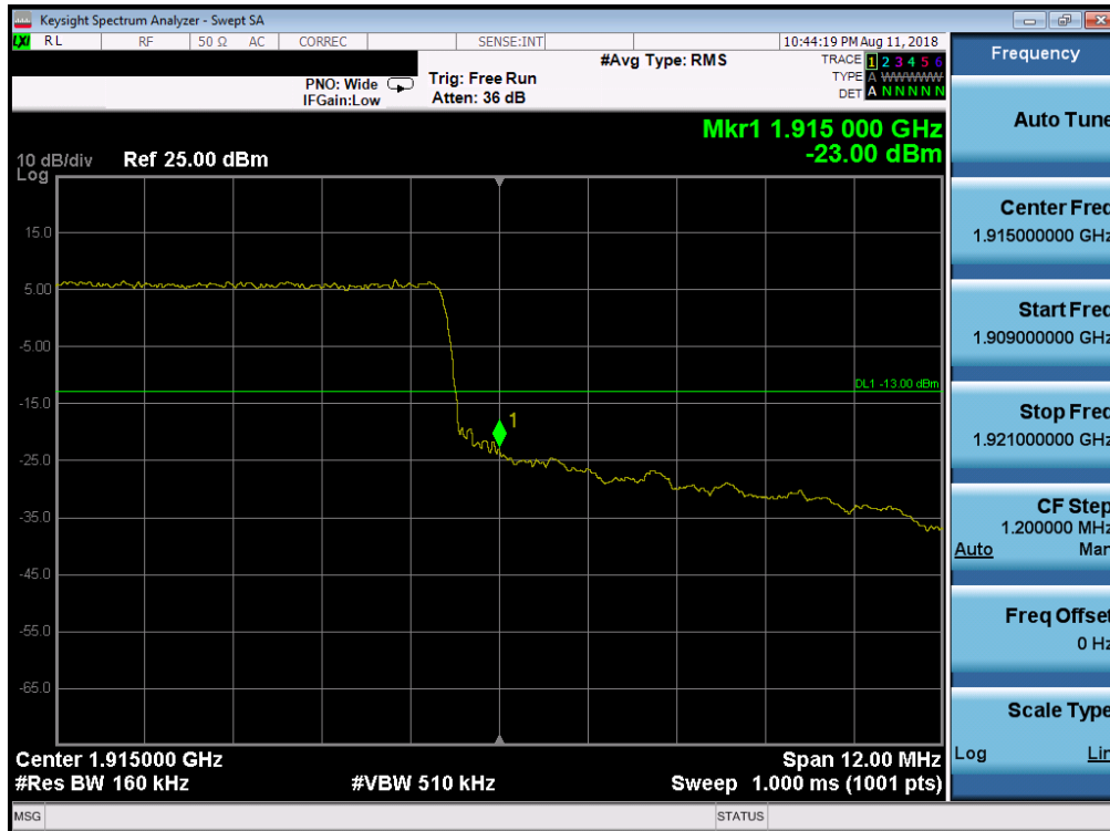
Plot 7-312. Upper Band Edge Plot (Band 25 – 15.0MHz QPSK – RB Size 75)
