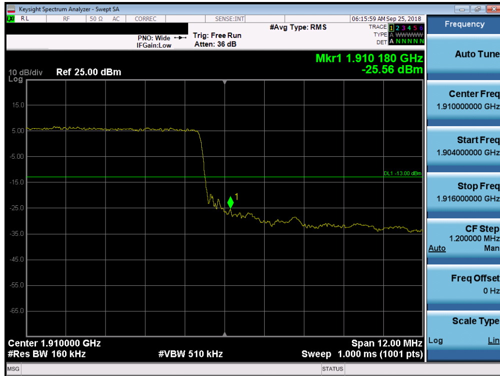
Plot 7-288. Upper Band Edge Plot (Band 2 – 15.0MHz QPSK – RB Size 75)
