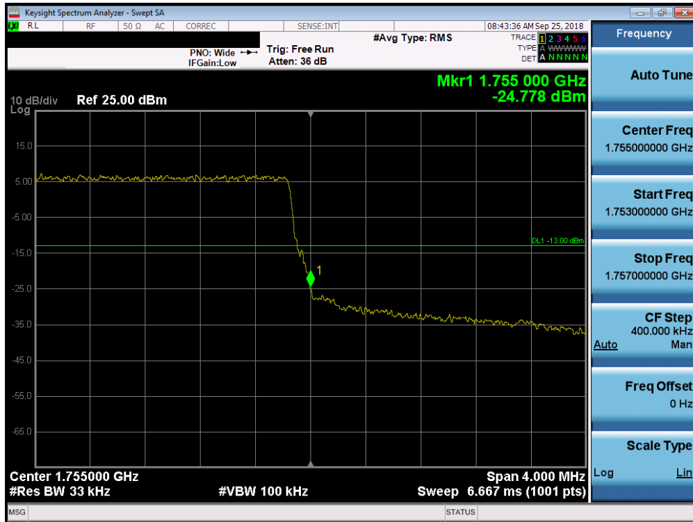
Plot 7-228. Upper Band Edge Plot (Band 4 – 3.0MHz QPSK – RB Size 15)
