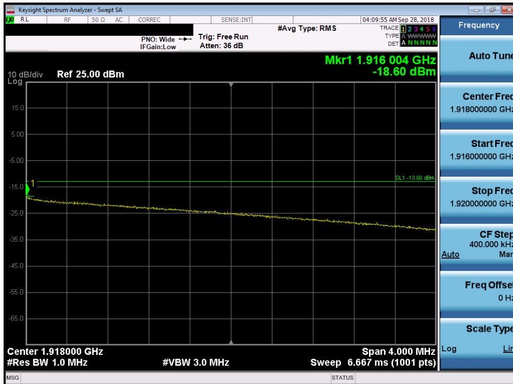
Plot 7-309. Upper Extended Band Edge Plot (Band 25 – 10.0MHz QPSK – RB Size 50)
