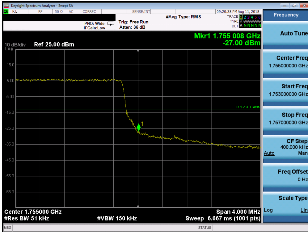
Plot 7-232. Upper Band Edge Plot (Band 4 – 5.0MHz QPSK – RB Size 25)
