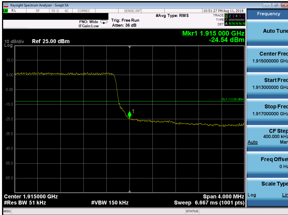
Plot 7-304. Upper Band Edge Plot (Band 25 – 5.0MHz QPSK – RB Size 25)
