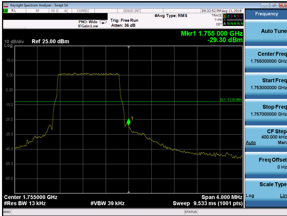
Plot 7-224. Upper Band Edge Plot (Band 4 – 1.4MHz QPSK – RB Size 6)
