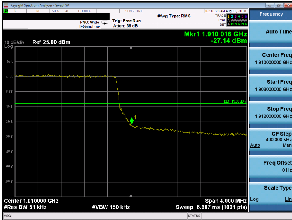
Plot 7-280. Upper Band Edge Plot (Band 2 – 5.0MHz QPSK – RB Size 25)
