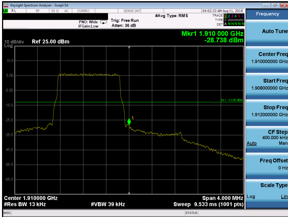
Plot 7-272. Upper Band Edge Plot (Band 2 – 1.4MHz QPSK – RB Size 6)
