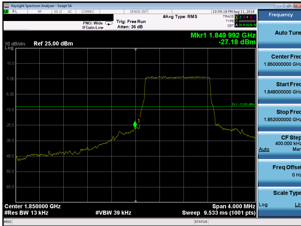
Plot 7-294. Lower Band Edge Plot (Band 25 – 1.4MHz QPSK – RB Size 6)
