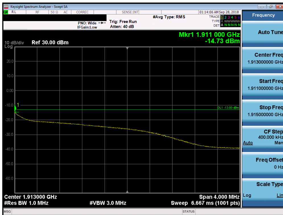
Plot 7-68. Extended Band Edge Plot (PCS WCDMA Mode - High Channel)
