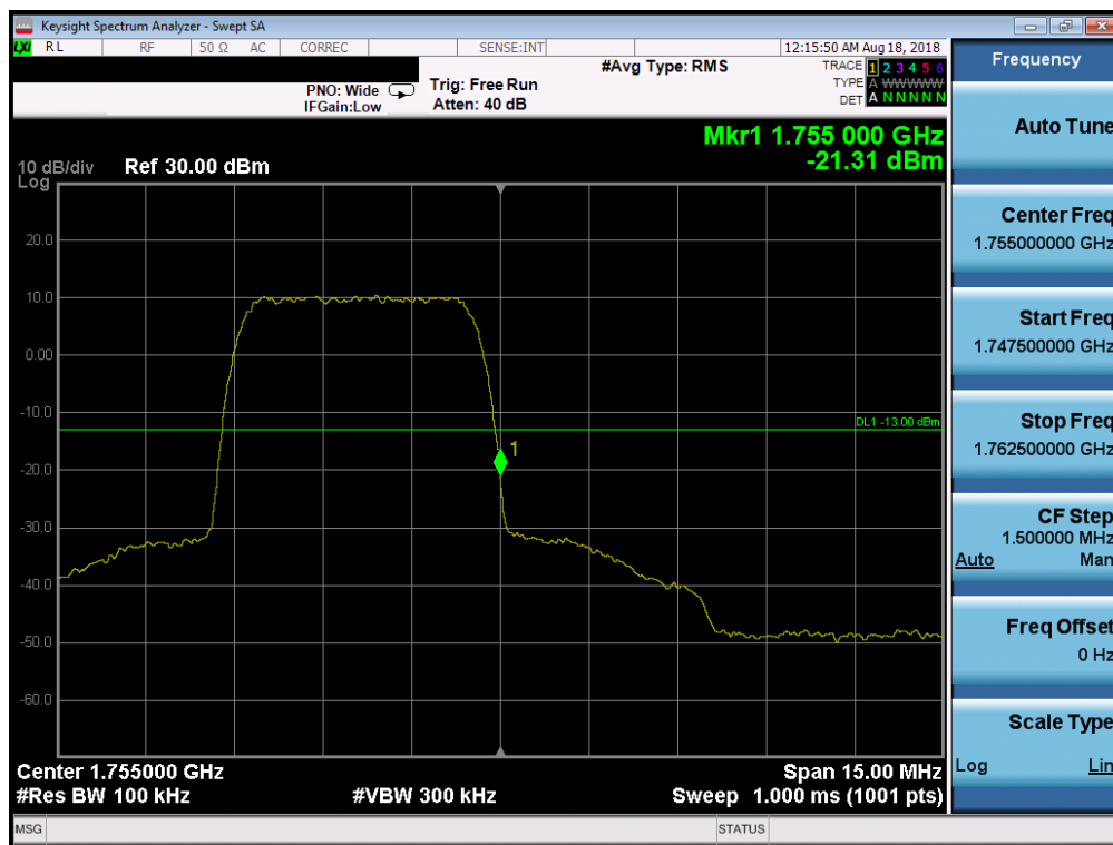
Plot 7-63. Band Edge Plot (AWS WCDMA Mode - High Channel)
