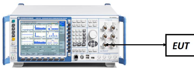
Figure 7-5. ERP/EIRP Measurement Setup
