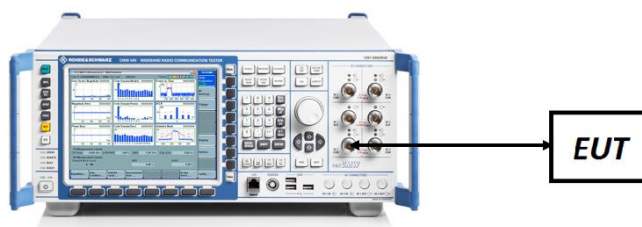
Figure 7-5. ERP/EIRP Measurement Setup
