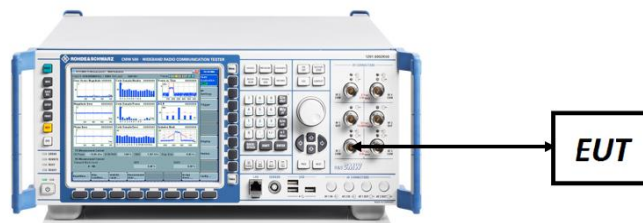
Figure 7-4. Conducted Power Measurement Setup
