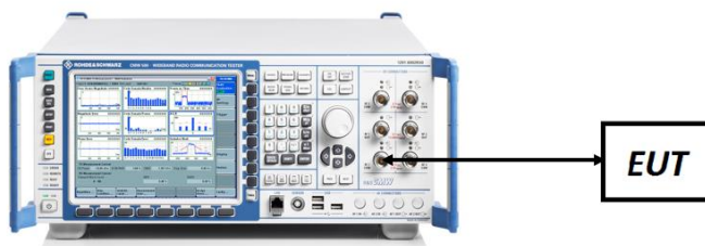
Figure 7-5. ERP/EIRP Measurement Setup
