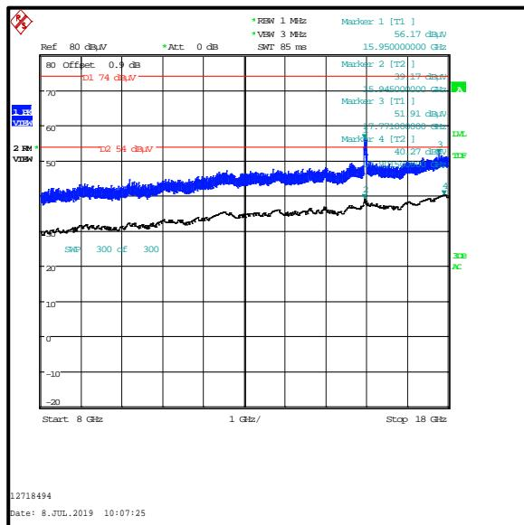
**Transmitter Out of Band Radiated Emissions - *Bluetooth LE bottom channel / 2.4 GHz WLAN (MIMO) top channel (continued)***
