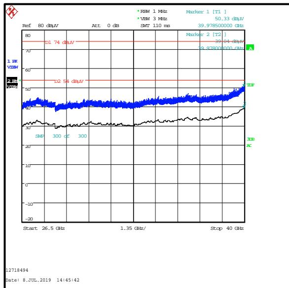
**4.2. Transmitter Out of Band Radiated Emissions - *Bluetooth Basic Rate top channel / 5 GHz WLAN (SISO) bottom channel*****Test Summary:**
