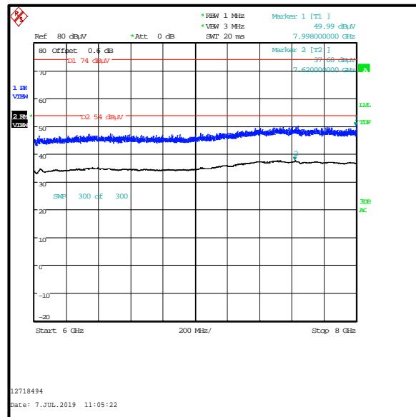
**Transmitter Out of Band Radiated Emissions - *Bluetooth Basic Rate bottom channel / 2.4 GHz WLAN (MIMO) top channel / 5 GHz WLAN (SISO) bottom channel (continued)***
