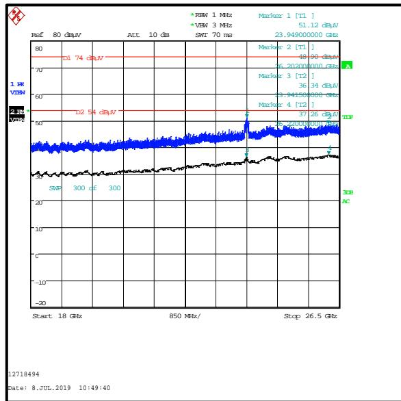
**4.11. Transmitter Out of Band Radiated Emissions - *Bluetooth Basic Rate bottom channel / 2.4 GHz WLAN (MIMO) top channel / 5 GHz WLAN (SISO) bottom channel*****Test Summary:**
