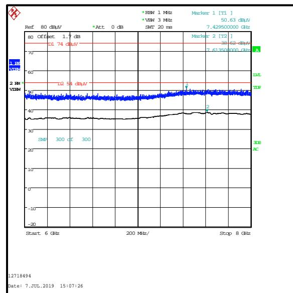
**Transmitter Out of Band Radiated Emissions - *Bluetooth Basic Rate bottom channel / 5 GHz WLAN (SISO) top channel (continued)***
