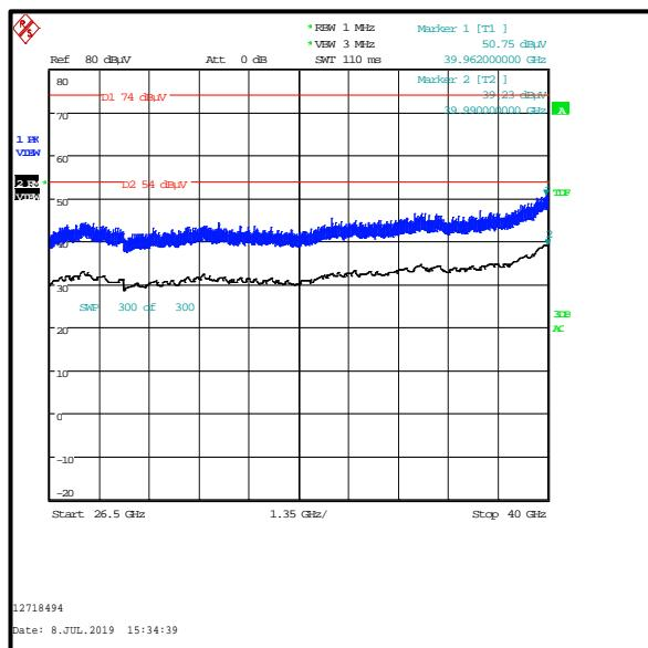
**4.7. Transmitter Out of Band Radiated Emissions - *Bluetooth Basic Rate bottom channel / 2.4 GHz WLAN (MIMO) top channel*****Test Summary:**
