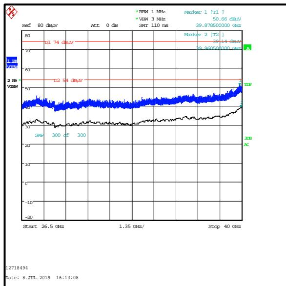
**4.13. Transmitter Out of Band Radiated Emissions - *Bluetooth Basic Rate top channel / 2.4 GHz WLAN (MIMO) bottom channel / 5 GHz WLAN (SISO) bottom channel*****Test Summary:**
