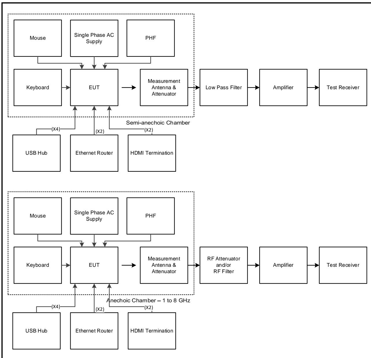
**Test Setup Diagrams (continued)****Test Setup for Transmitter Radiated Emissions (continued)**
