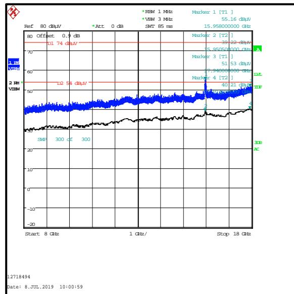
**Transmitter Out of Band Radiated Emissions - *Bluetooth Basic Rate bottom channel / 2.4 GHz WLAN (MIMO) top channel (continued)***
