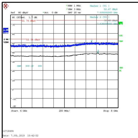
**Transmitter Out of Band Radiated Emissions - *Bluetooth Basic Rate bottom channel / 2.4 GHz WLAN (MIMO) top channel / 5 GHz WLAN (SISO) top channel (continued)***
