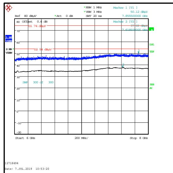
**Transmitter Out of Band Radiated Emissions - 2.4 GHz WLAN (MIMO) top channel / 5 GHz WLAN (SISO) bottom channel (continued)**
