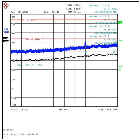
**4.8. Transmitter Out of Band Radiated Emissions - *Bluetooth Basic Rate top channel / 2.4 GHz WLAN (MIMO) bottom channel*****Test Summary:**
