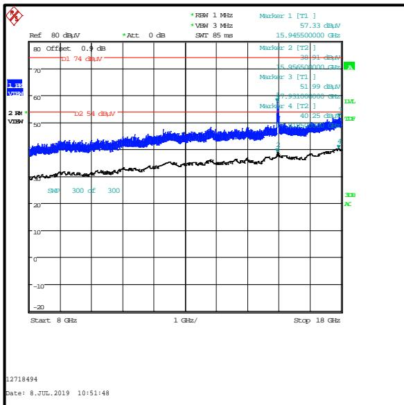
**4.12. Transmitter Out of Band Radiated Emissions - *Bluetooth Basic Rate bottom channel / 2.4 GHz WLAN (MIMO) top channel / 5 GHz WLAN (SISO) top channel*****Test Summary:**
