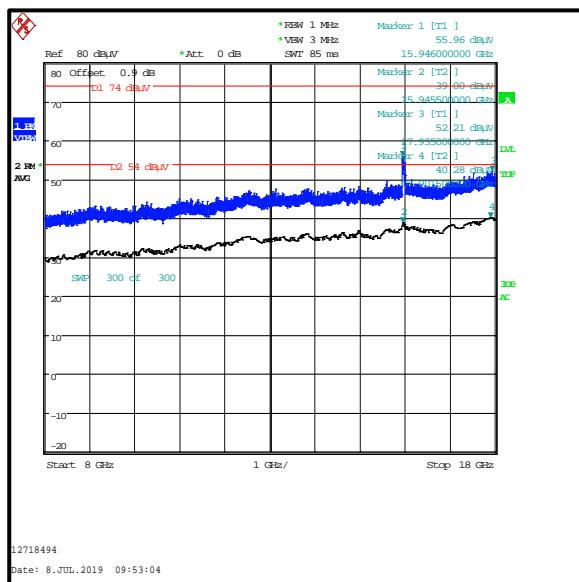
**Transmitter Out of Band Radiated Emissions - *Bluetooth Basic Rate top channel / 2.4 GHz WLAN (MIMO) bottom channel (continued)***
