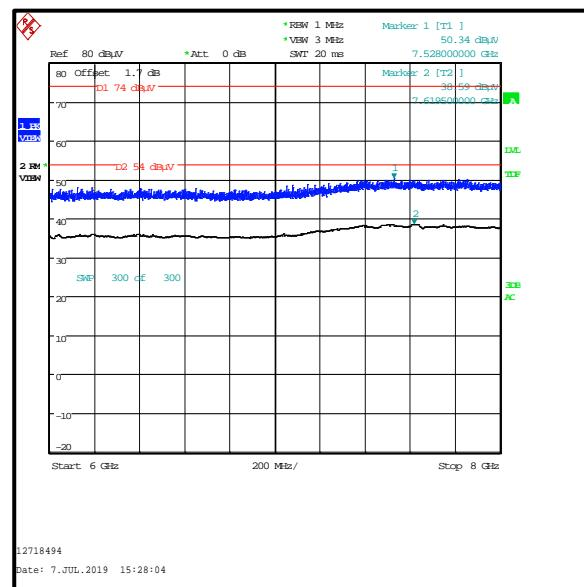
**Transmitter Out of Band Radiated Emissions - 2.4 GHz WLAN (MIMO) bottom channel / 5 GHz WLAN (SISO) top channel (continued)**
