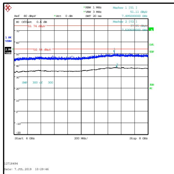
**Transmitter Out of Band Radiated Emissions - *Bluetooth Basic Rate top channel / 5 GHz WLAN (SISO) bottom channel (continued)***
