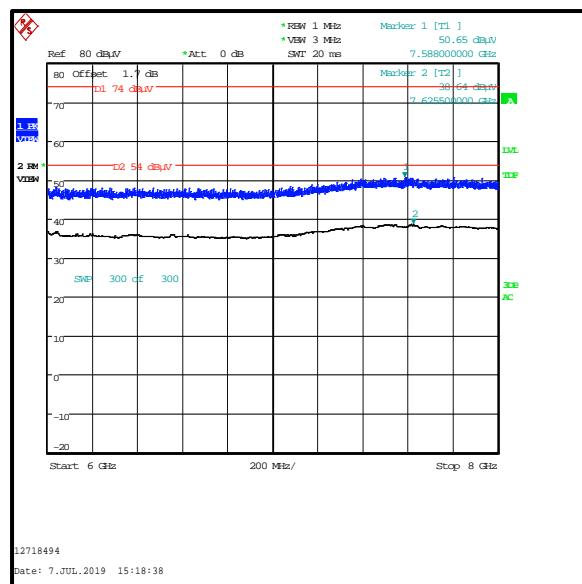
**Transmitter Out of Band Radiated Emissions - *Bluetooth LE bottom channel / 5 GHz WLAN (SISO) top channel (continued)***
