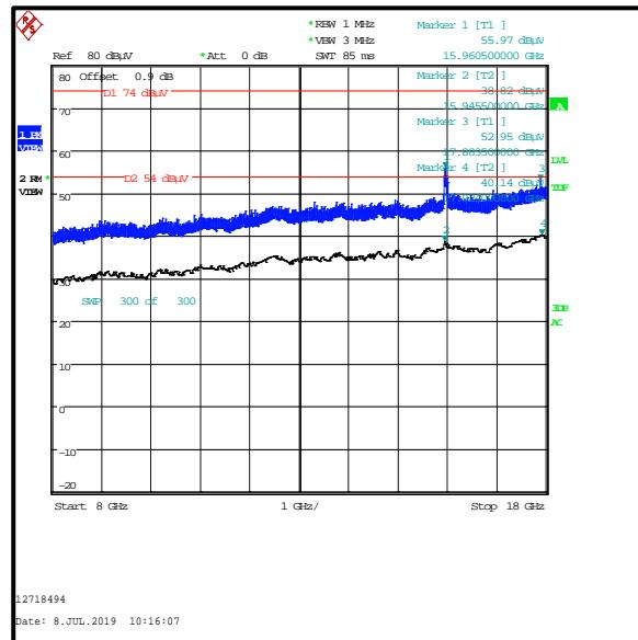
**Transmitter Out of Band Radiated Emissions - *Bluetooth LE top channel / 2.4 GHz WLAN (MIMO) bottom channel (continued)***
