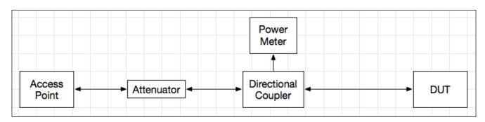
Verification checks have been performed to demonstrate Body Detect Mode. Conducted power spot check measurements have been taken on each frequency band for a given configuration mode, when Body Detect Mode is enabled and disabled. Body Detect Mode is described in detail within the technical description of the device.
