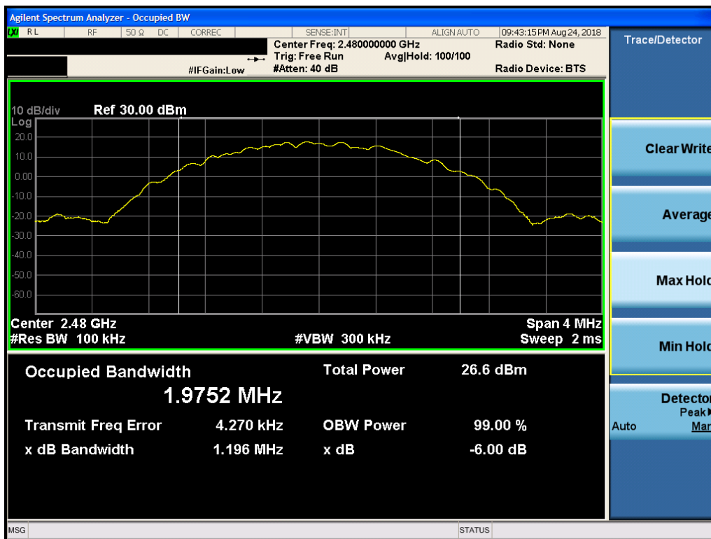
Plot 7-18. 6dB Bandwidth Plot (Bluetooth (LE), 2Mbps, ePA – Ch. 39, Antenna 2)
