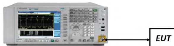
Figure 7-1. Test Instrument & Measurement Setup
