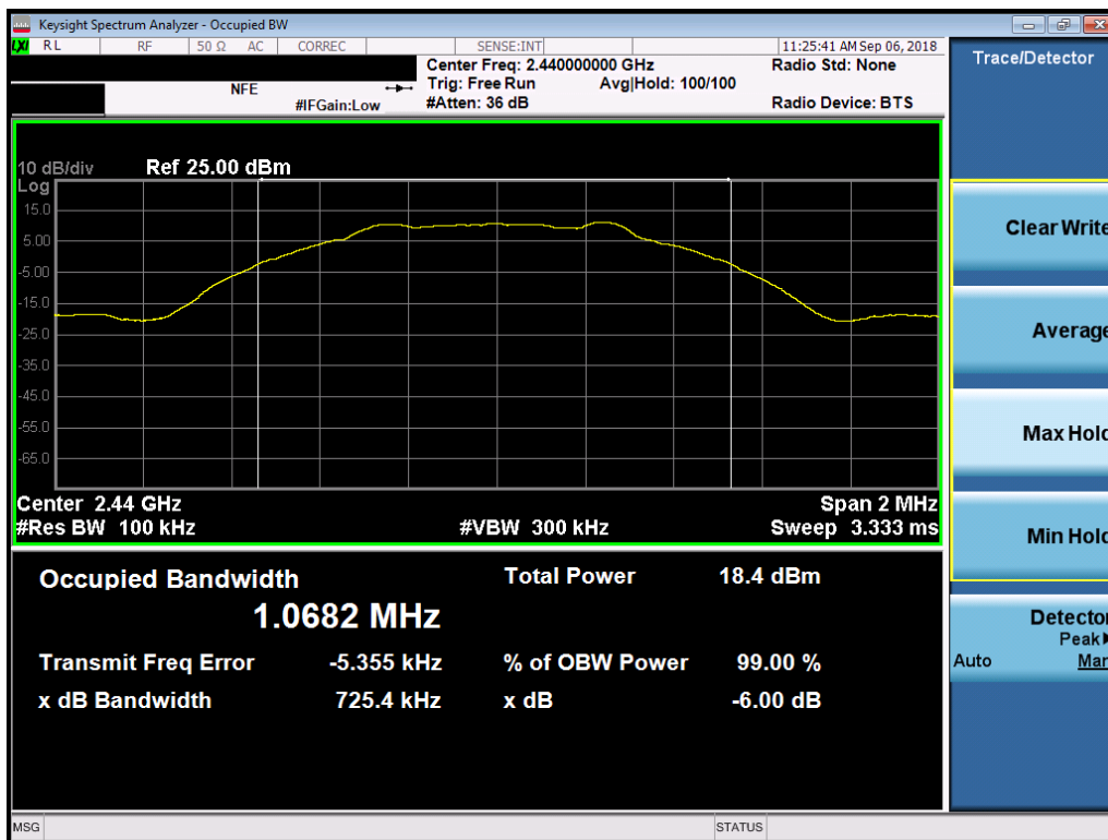
Plot 7-14. 6dB Bandwidth Plot (Bluetooth (LE), 1Mbps, ePA – Ch. 19, Antenna 2)
