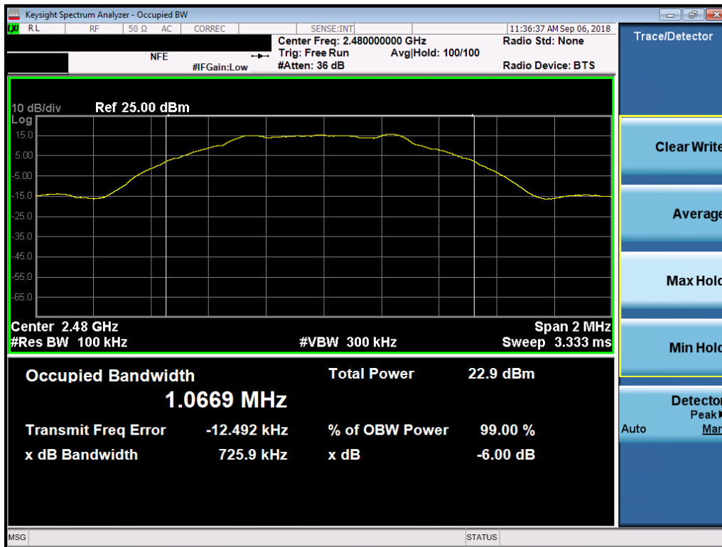
Plot 7-15. 6dB Bandwidth Plot (Bluetooth (LE), 1Mbps, ePA – Ch. 39, Antenna 2)
