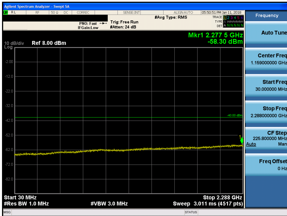
Plot 7-164. Conducted Spurious Plot (Band 30 - 5.0MHz QPSK - RB Size 1, RB Offset 0 - Mid Channel)
