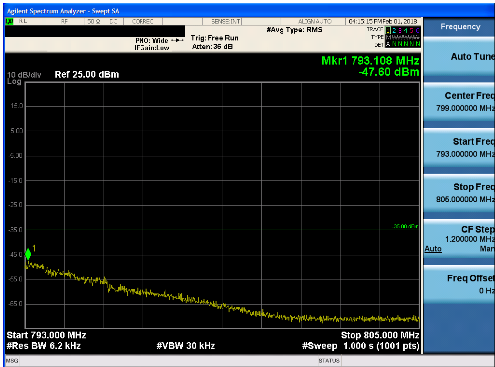
Plot 7-207. Upper Emission Mask Edge Plot (Band 13 - 10.0MHz QPSK - Full RB Configuration)
