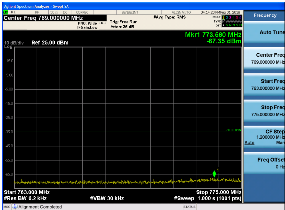
Plot 7-205. Lower Emission Mask Edge Plot (Band 13 - 10.0MHz QPSK - Full RB Configuration)
