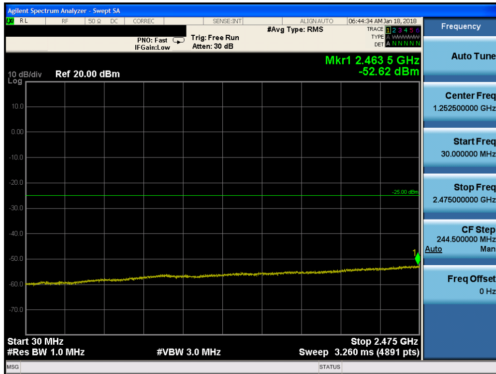
Plot 7-170. Conducted Spurious Plot (Band 7 - 20.0MHz QPSK - RB Size 1, RB Offset 0 - Low Channel)
