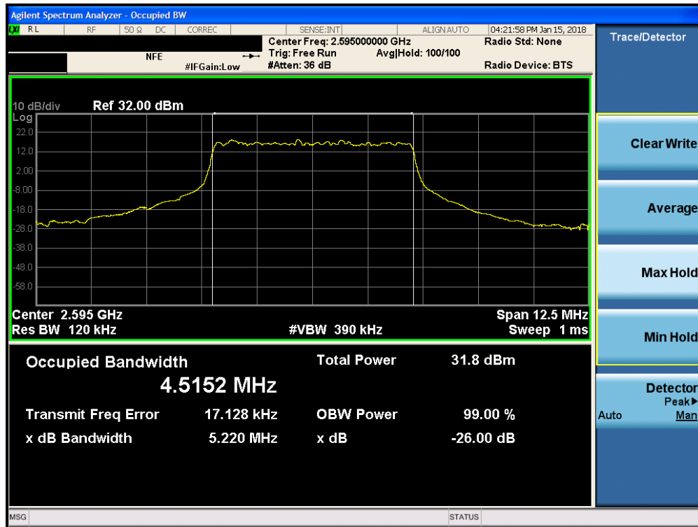
Plot 7-81. Occupied Bandwidth Plot (Band 41 - 5.0MHz QPSK - Full RB Configuration)
