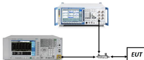
Figure 7-4. Test Instrument & Measurement Setup
