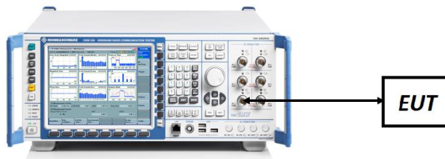
Figure 7-5. ERP/EIRP Measurement Setup
