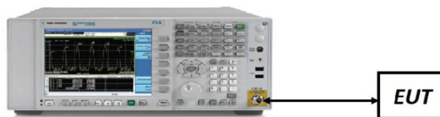
Figure 7-2. Test Instrument & Measurement Setup
