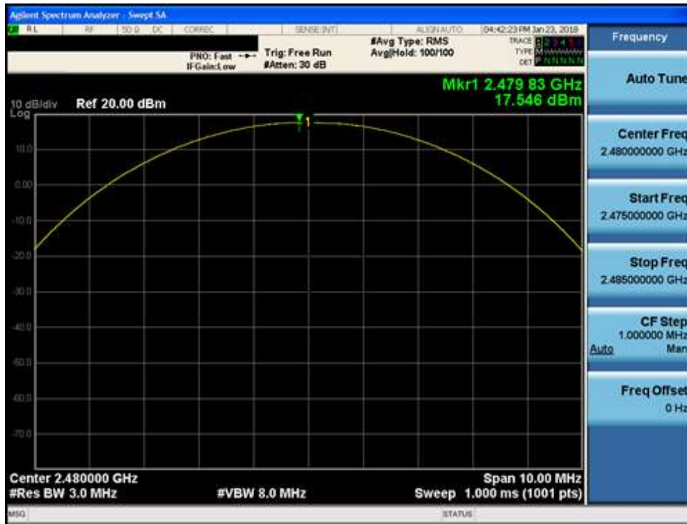
Plot 7-15. Peak Conducted Power (GFSK, ePA – Ch. 78)
