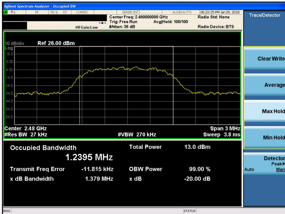
Plot 7-12. 20dB Bandwidth Plot (Bluetooth, 8DPSK, iPA – Ch. 78)
