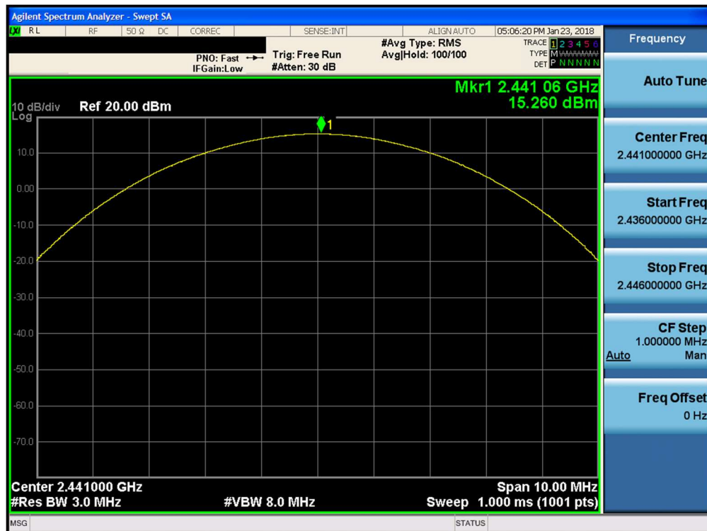
Plot 7-20. Peak Conducted Power (8DPSK, ePA – Ch. 39)
