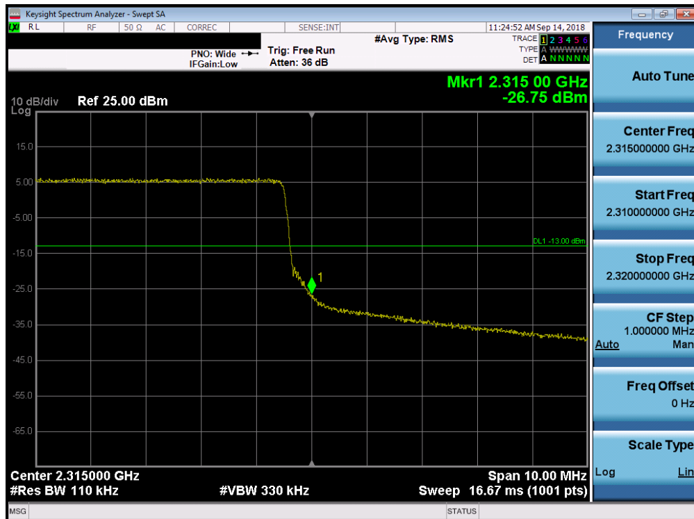
Plot 7-302. Upper Band Edge Plot (Band 30 – 10.0MHz QPSK – RB Size 50)
