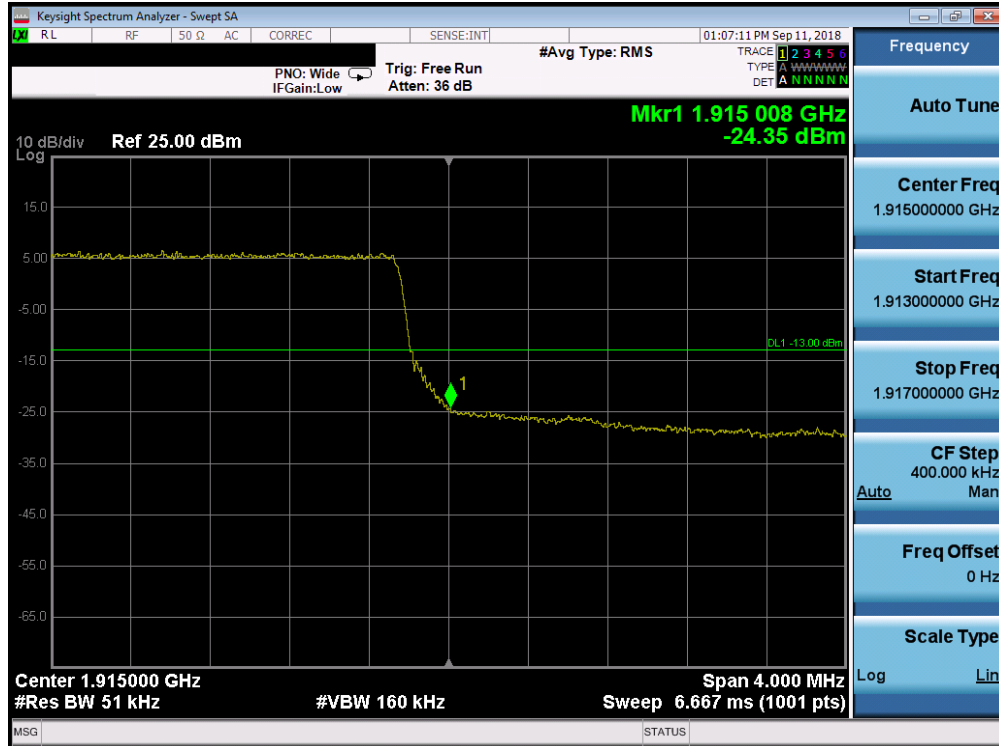
Plot 7-281. Upper Band Edge Plot (Band 25 – 5.0MHz QPSK – RB Size 25)
