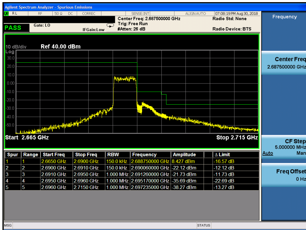
Plot 7-313. Upper ACP Plot (Band 41 – 5.0MHz QPSK – RB Size 25)
