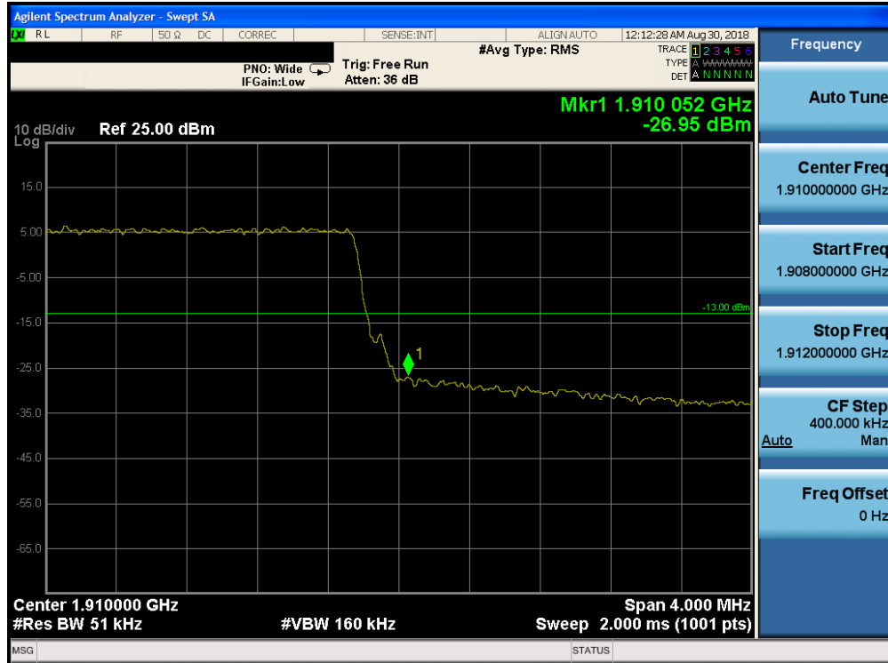
Plot 7-257. Upper Band Edge Plot (Band 2 – 5.0MHz QPSK – RB Size 25)
