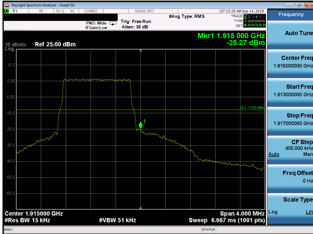
Plot 7-273. Upper Band Edge Plot (Band 25 – 1.4MHz QPSK – RB Size 6)
