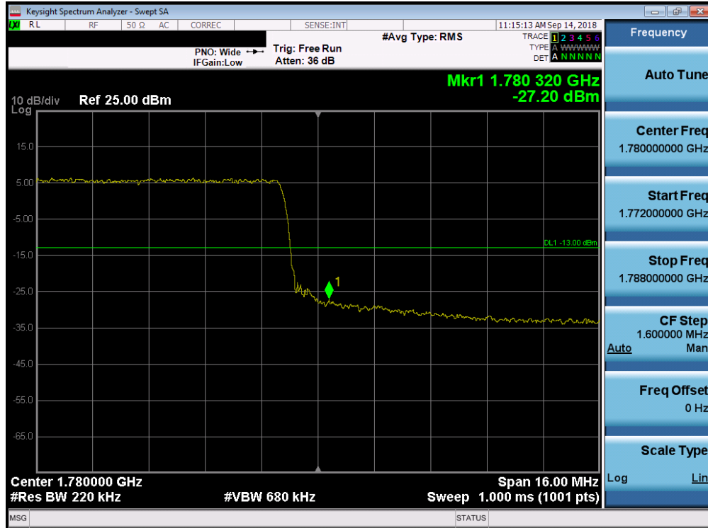
Plot 7-245. Upper Band Edge Plot (Band 66 – 20.0MHz QPSK – RB Size 100)
