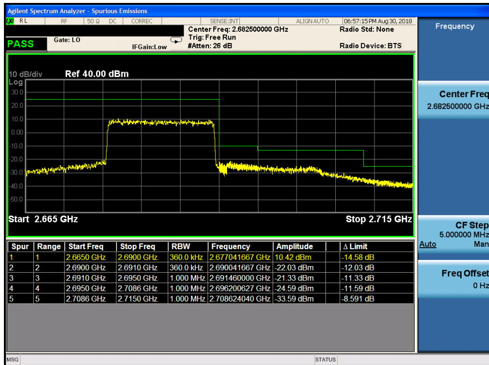
Plot 7-317. Upper ACP Plot (Band 41 – 15.0MHz QPSK – RB Size 75)
