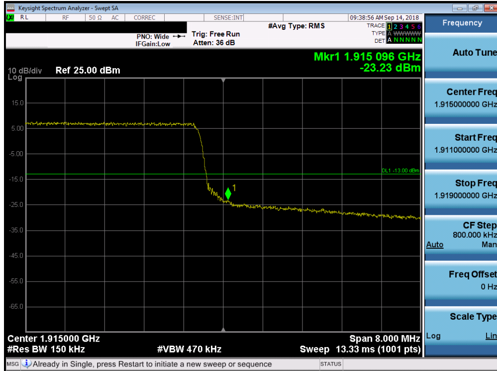
Plot 7-285. Upper Band Edge Plot (Band 25 – 10.0MHz QPSK – RB Size 50)
