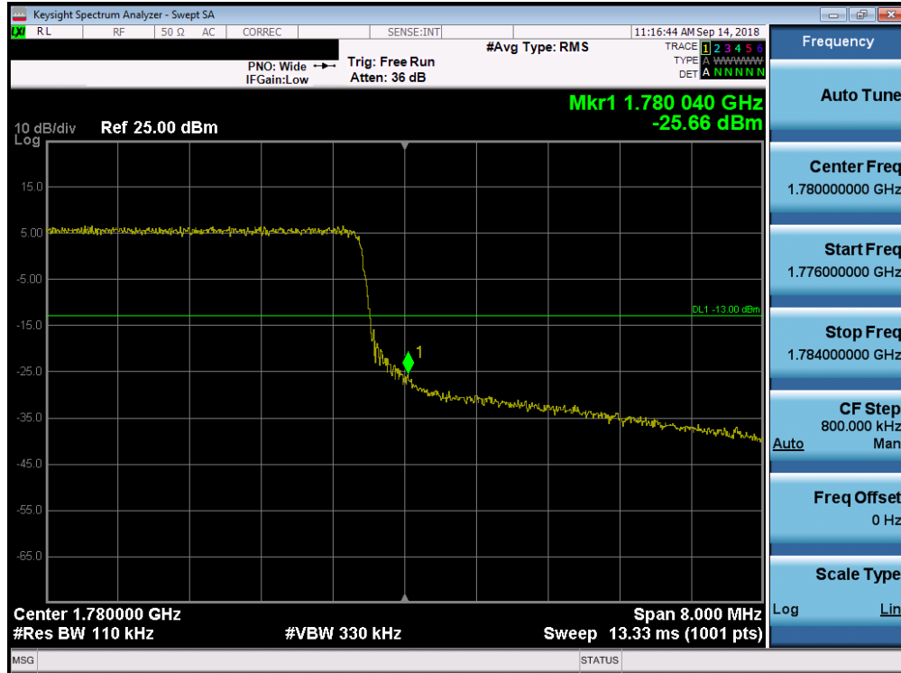
Plot 7-237. Upper Band Edge Plot (Band 66 – 10.0MHz QPSK – RB Size 50)
