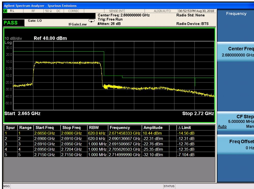
Plot 7-319. Upper ACP Plot (Band 41 – 20.0MHz QPSK – RB Size 100)
