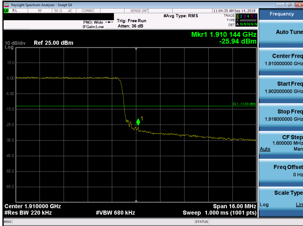
Plot 7-269. Upper Band Edge Plot (Band 2 - 20.0MHz QPSK - RB Size 100)
