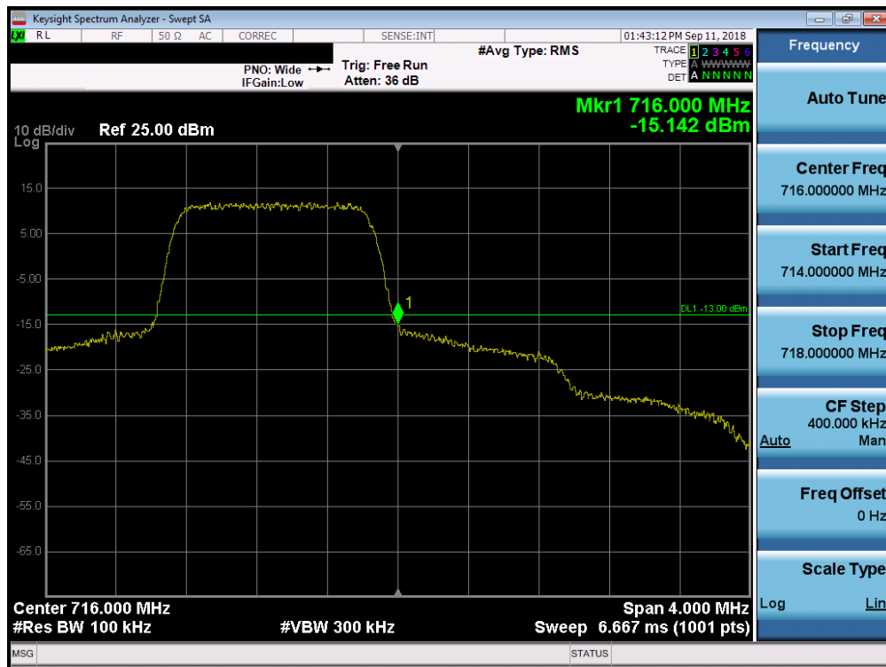
Plot 7-164. Upper Band Edge Plot (Band 12 – 1.4MHz QPSK – RB Size 6)
