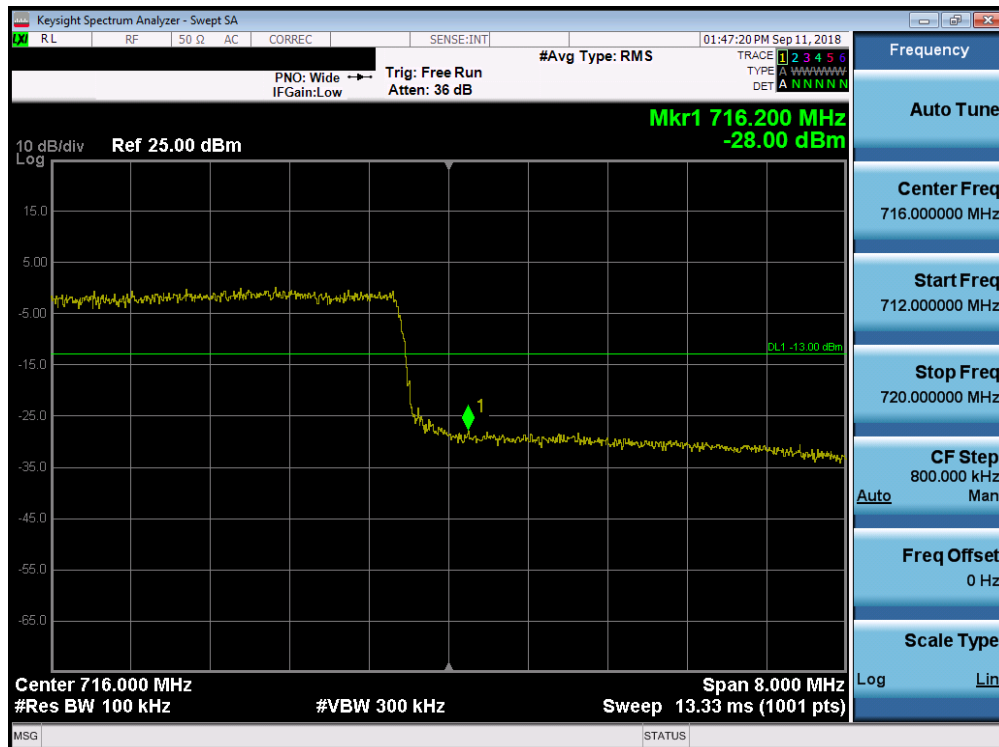
Plot 7-174. Upper Band Edge Plot (Band 17 – 10.0MHz QPSK – RB Size 50)
