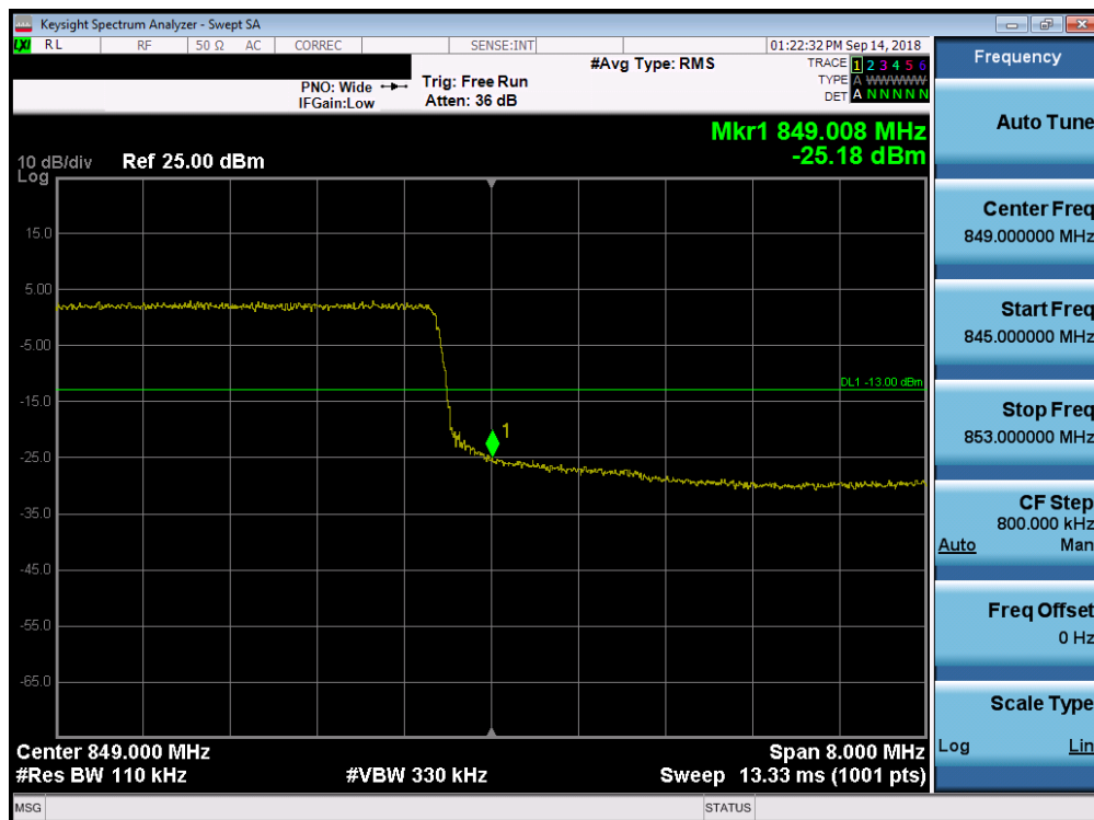
Plot 7-198. Upper Band Edge Plot (Band 26 – 10.0MHz QPSK – RB Size 50)
