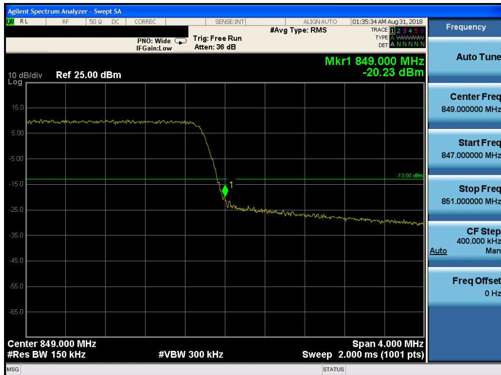
Plot 7-196. Upper Band Edge Plot (Band 26 – 5.0MHz QPSK – RB Size 25)
