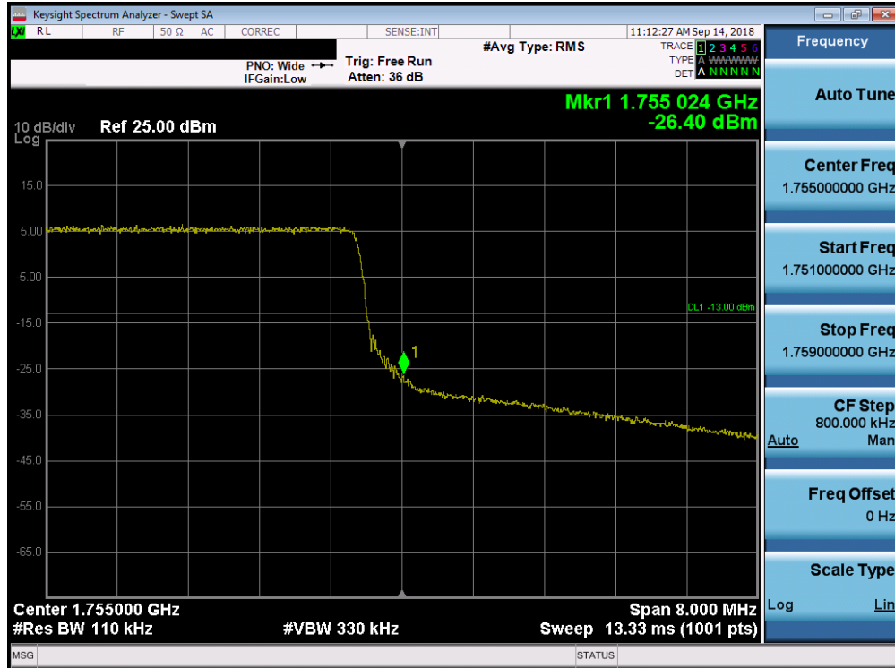
Plot 7-213. Upper Band Edge Plot (Band 4 – 10.0MHz QPSK – RB Size 50)
