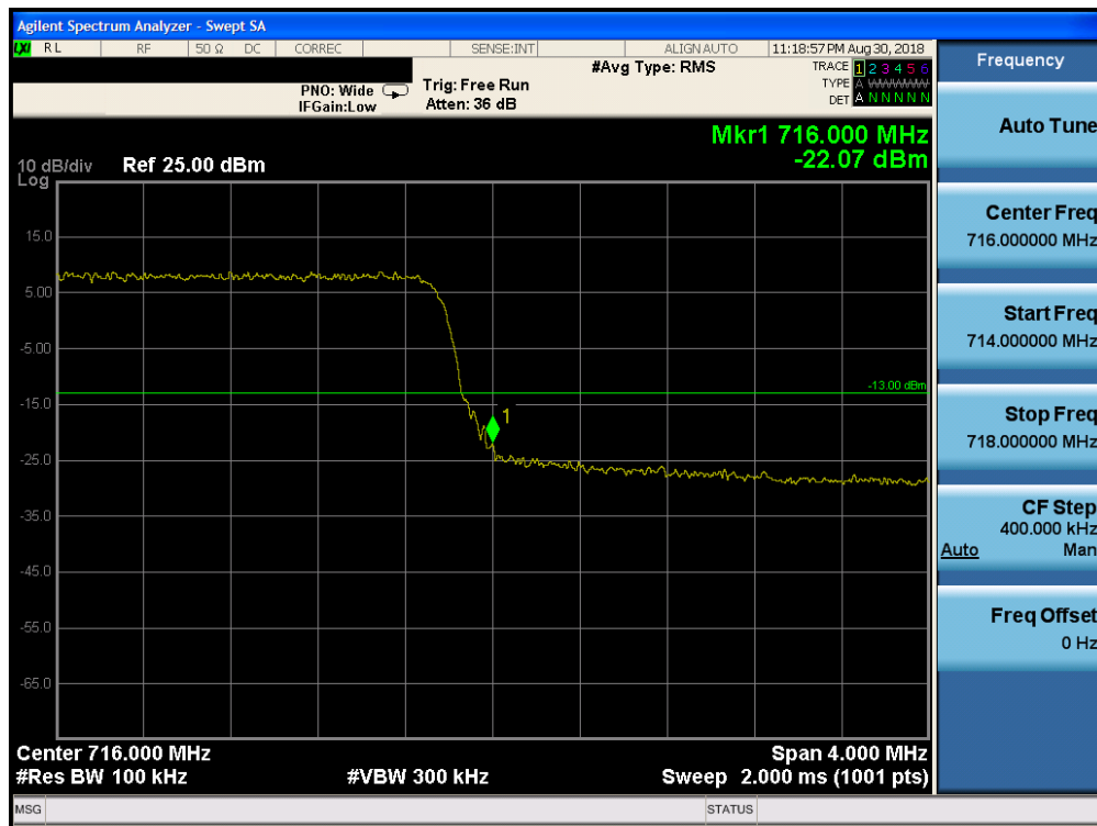
Plot 7-172. Upper Band Edge Plot (Band 17 – 5.0MHz QPSK – RB Size 25)
