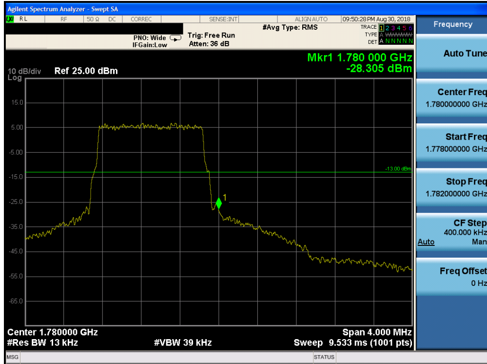
Plot 7-225. Upper Band Edge Plot (Band 66 – 1.4MHz QPSK – RB Size 6)
