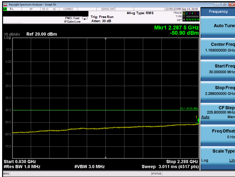
Plot 7-142. Conducted Spurious Plot (Band 30 – 10.0MHz QPSK – RB Size 1, RB Offset 0 – Mid Channel)
