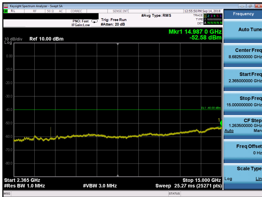
Plot 7-143. Conducted Spurious Plot (Band 30 – 10.0MHz QPSK – RB Size 1, RB Offset 0 – Mid Channel)
