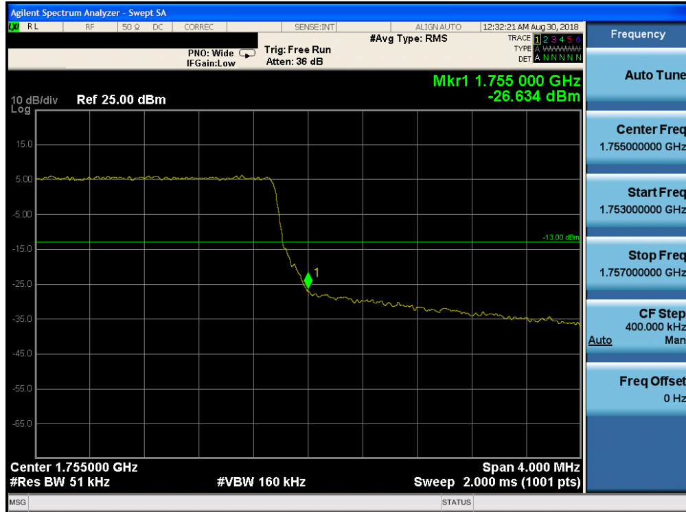
Plot 7-209. Upper Band Edge Plot (Band 4 – 5.0MHz QPSK – RB Size 25)
