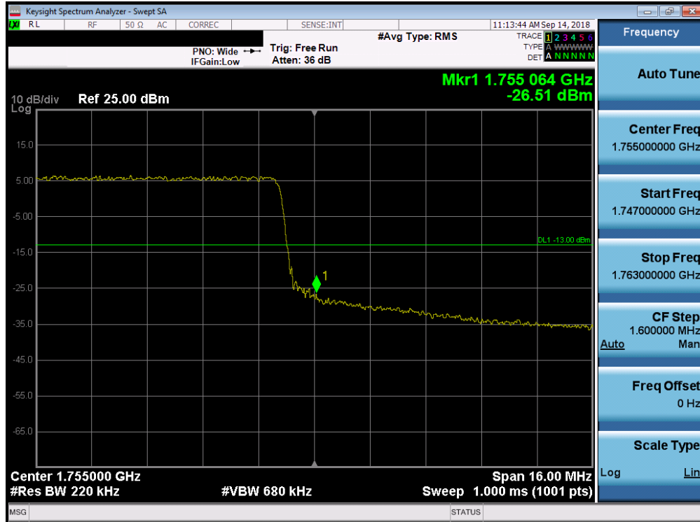
Plot 7-221. Upper Band Edge Plot (Band 4 – 20.0MHz QPSK – RB Size 100)
