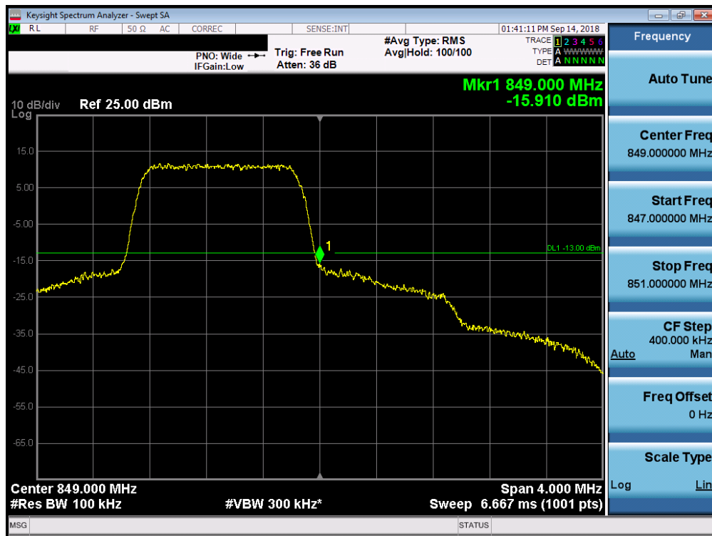
Plot 7-192. Upper Band Edge Plot (Band 26 – 1.4MHz QPSK – RB Size 6)
