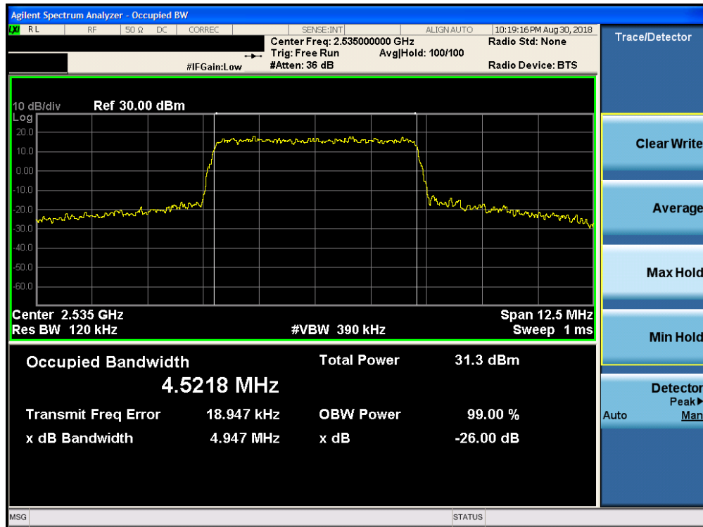
Plot 7-73. Occupied Bandwidth Plot (Band 7 – 5.0MHz QPSK – RB Size 25)
