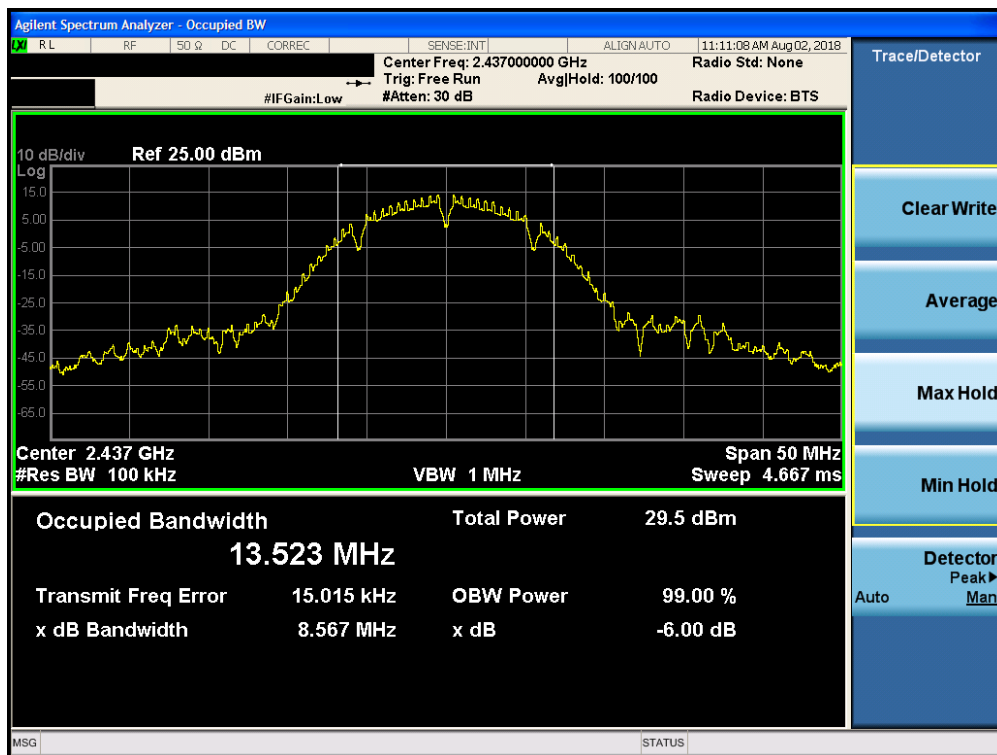
Plot 7-2. 6dB Bandwidth Plot SISO CORE0 (802.11b – Ch. 6)
