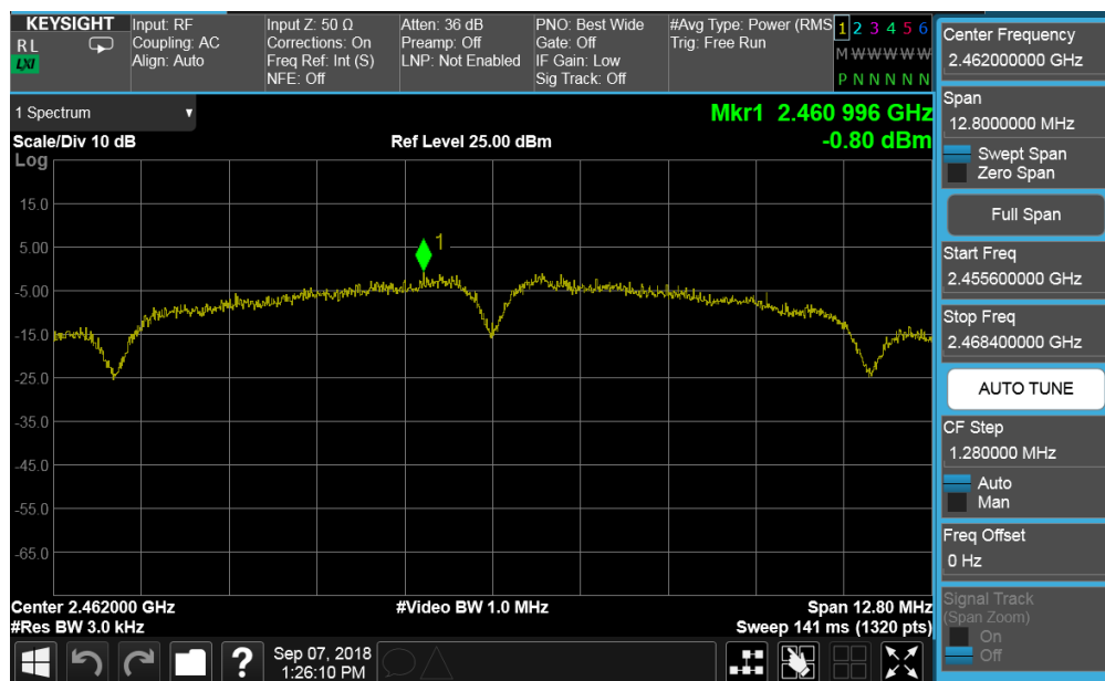
Plot 7-30. Power Spectral Density Plot SISO CORE0 (802.11b – Ch. 11)
