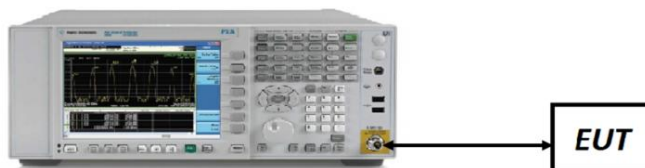
Figure 7-3. Test Instrument & Measurement Setup
